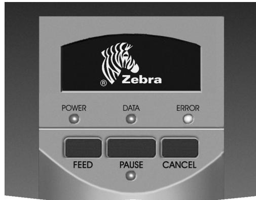
Figure 11. Standard Front Panel
