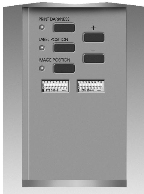
Figure 16. Standard Front Panel
