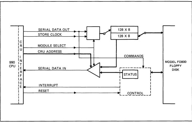
Figure 3. Floppy-Disk Controller, Simplified Diagram
