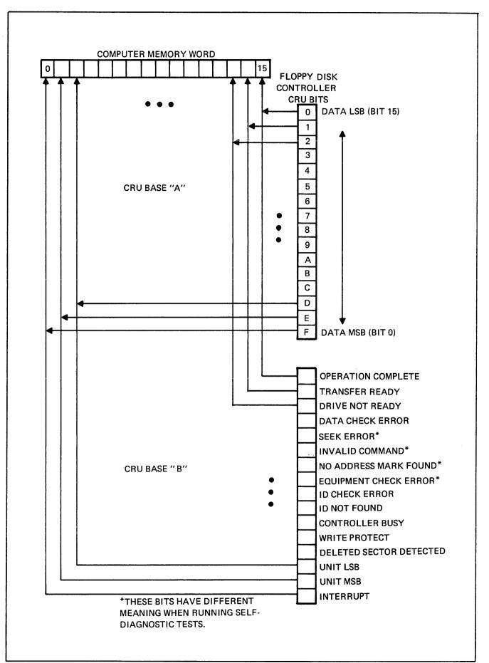
Figure 4. CRU Input Format (Controller to Computer)
