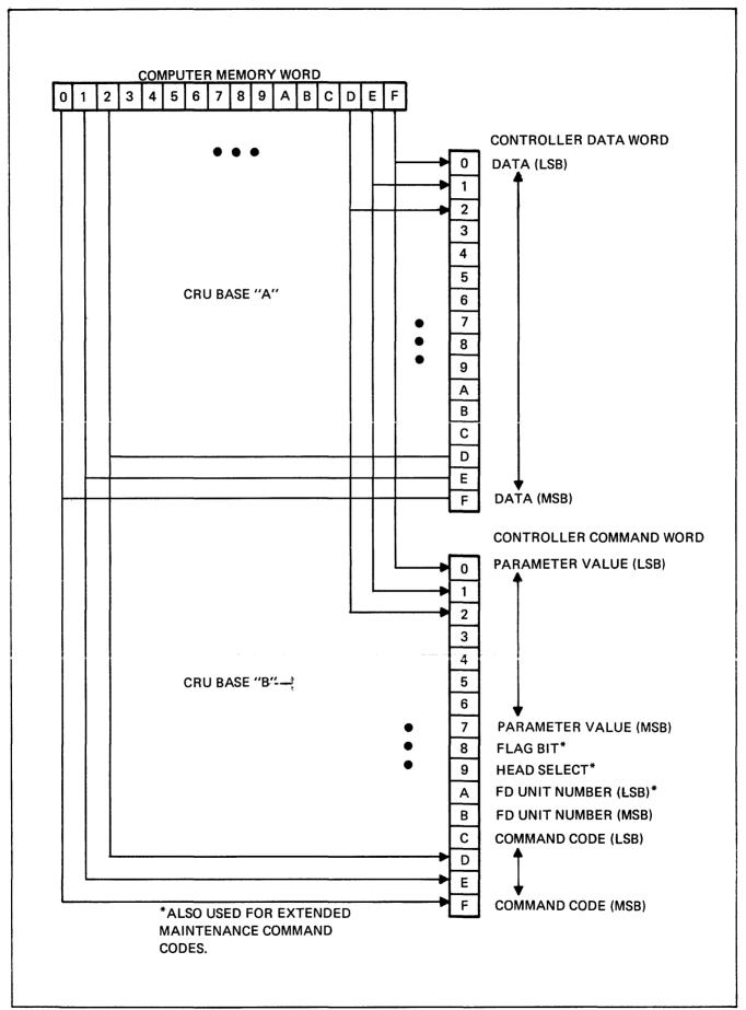
Figure 5. CRU Output Format (Computer to Controller)
