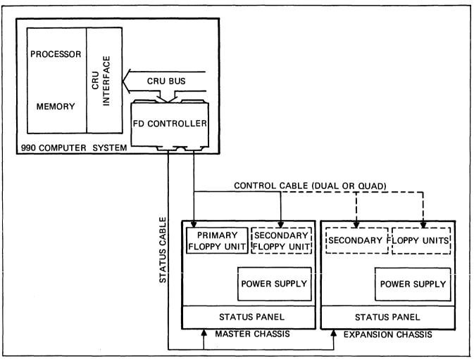
Figure 2. Floppy-Disk System Configuration
