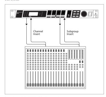
Fig. 4.2: Wiring the VIRTUALIZER PRO in the insert path
