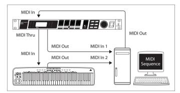
Fig. 4.4: VIRTUALIZER PRO in MIDI connection with a sequencer (computer) and a keyboard
