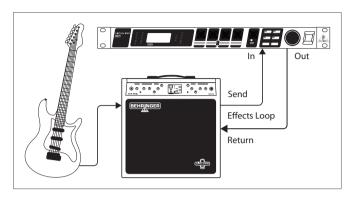
Fig. 4.3: Connecting the VIRTUALIZER PRO to a guitar amp (send/return mono)
