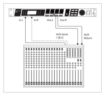
Fig. 4.1: Wiring aux busses
