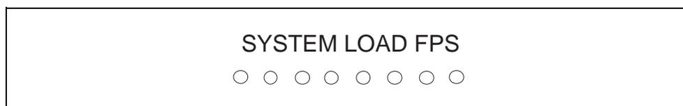
The eight lamps give a real-time indication of the volume of traffic in frames per second. If there is no traffic on the backplane of the WaveSwitch 100, none of the lamps comes on.
