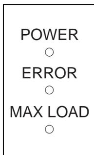
The POWER lamp indicates that the internal power supply is providing electrical power to the circuit boards in the unit.
