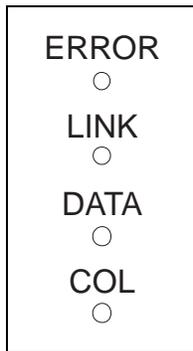
If four adjacent ERROR indicator lamps come on and stay on, an error was detected on the bridge-circuit ASIC that controls that group of ports. For the sixteen-port base unit, the port groups are: 1-4, 5-8, 9-12, and 13-16.
