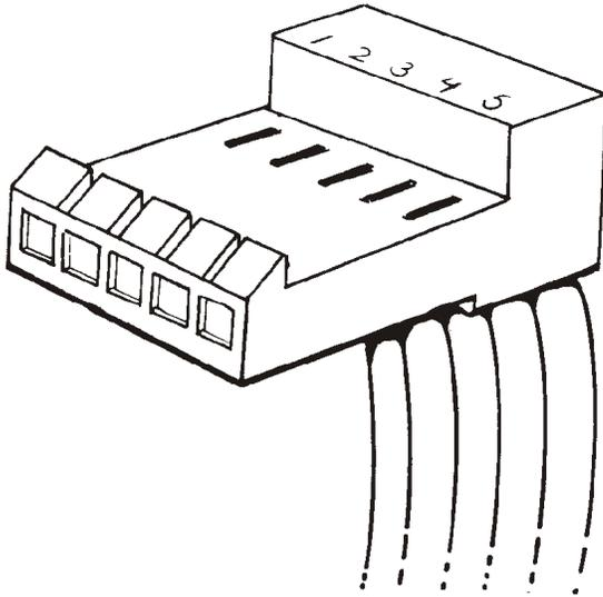
**(h)** Turn power off. Reconnect 5-pin ribbon cable and 2-pin plug. Turn power on and remeasure voltage at +5.65 volt connector pin. Meter should read 5.45 - 5.85 VDC. If voltage is not within limits, turn off power and measure resistance of R2 (Figure 5). If OK, replace logic board. If not OK, troubleshoot power supply board.
