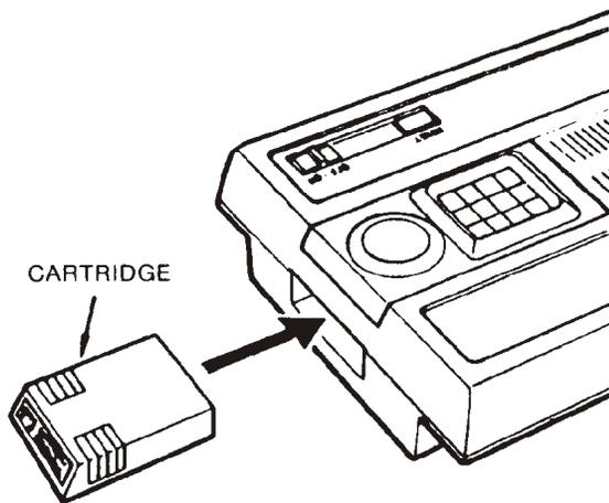
3. Insert the MTE-201 Test Cartridge. Slide the ON/OFF Switch to the ON position and depress the Reset Button on the Master Component. The unit will proceed through a series of checks.
