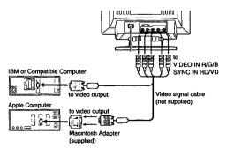
Note: Use HD15 (Female)-HD15(Male without No.9 pin) adapter (supplied) for current DOS computer which has no compliance of DDC 2AB and its No 9 pin is disconnected
