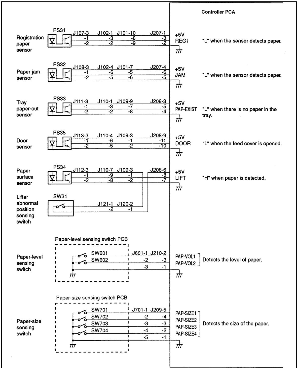
Figure 7-36 2000-Sheet Input Unit Controller PCA Inputs
