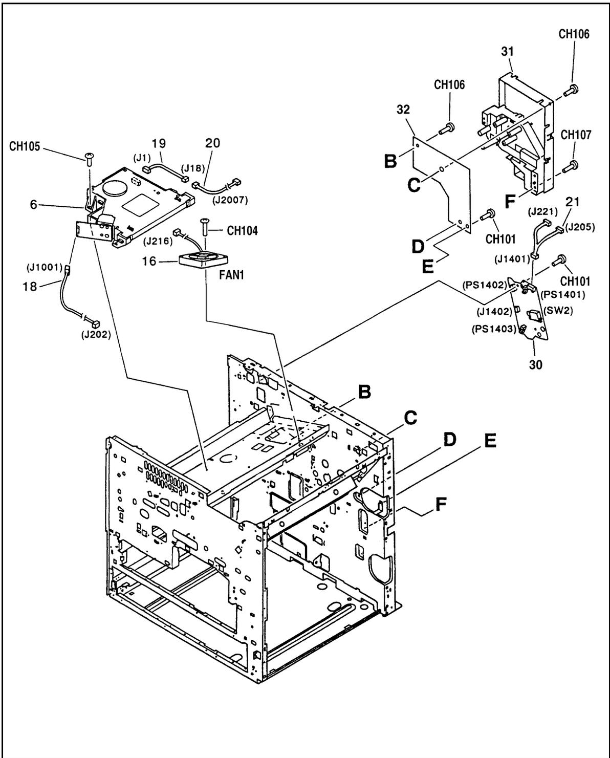
Figure 8-5 Printer Internal Components (3 of 4)
