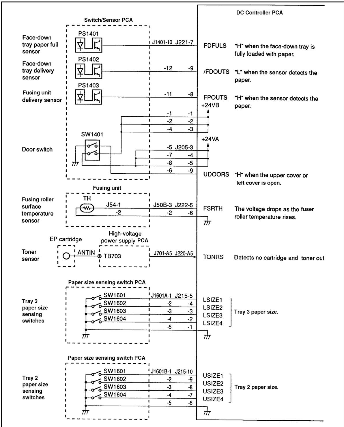
Figure 7-31 DC Controller Inputs and Outputs (2 of 5)
