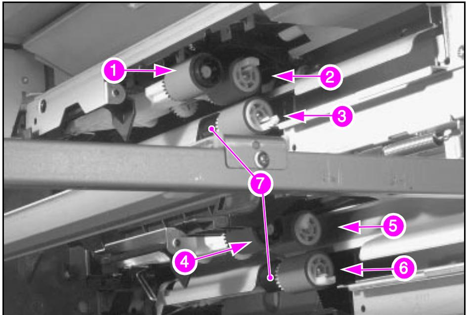
Tray 2 and 3, Pickup, Feed, and Separation Rollers
