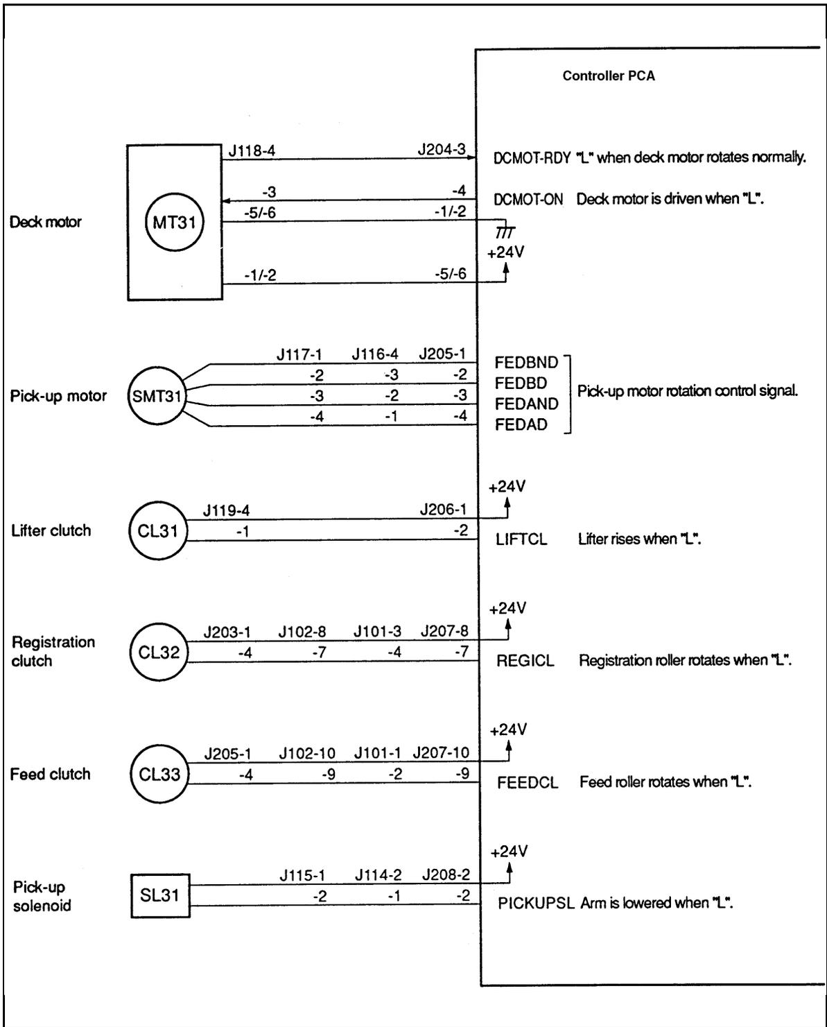
Figure 7-37 2000-Sheet Input Unit Controller PCA Outputs
