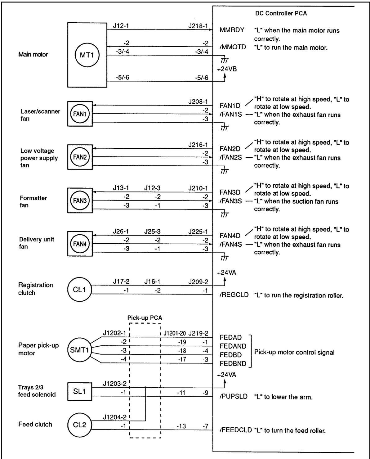
Figure 7-33 DC Controller Inputs and Outputs (4 of 5)
