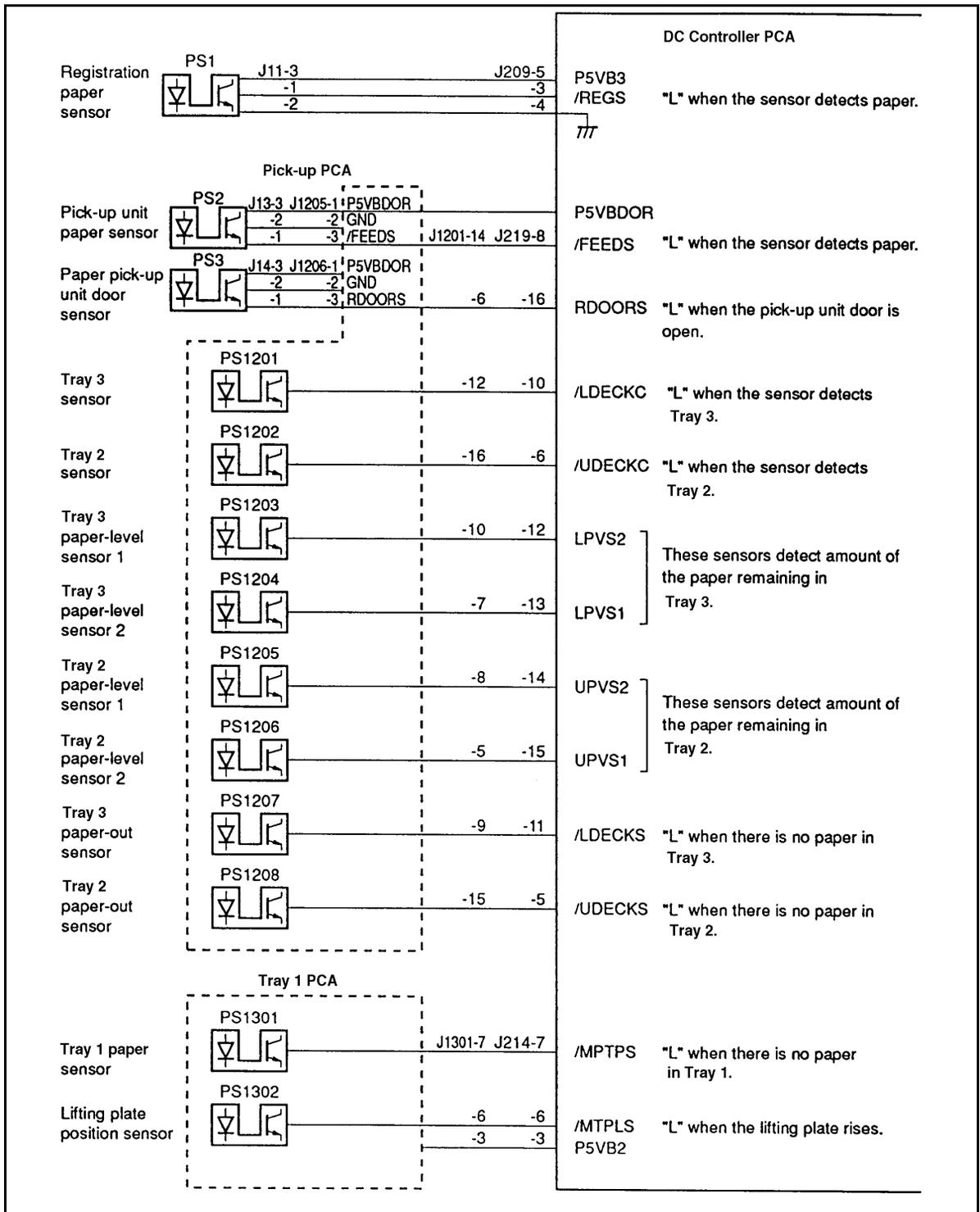
Figure 7-30 DC Controller Inputs and Outputs (1 of 5)
