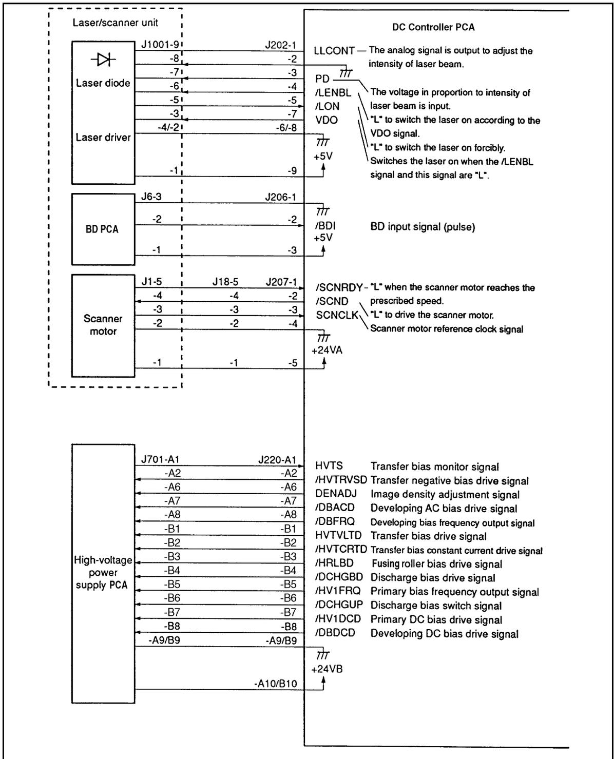
Figure 7-32 DC Controller Inputs and Outputs (3 of 5)
