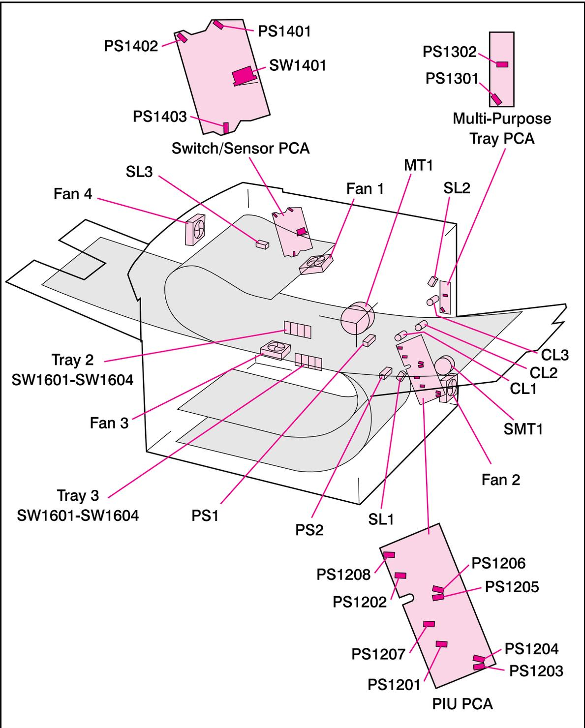
**Figure 5-15** Printer Sensors, Solenoids, Clutches, Motors, and Fans.
