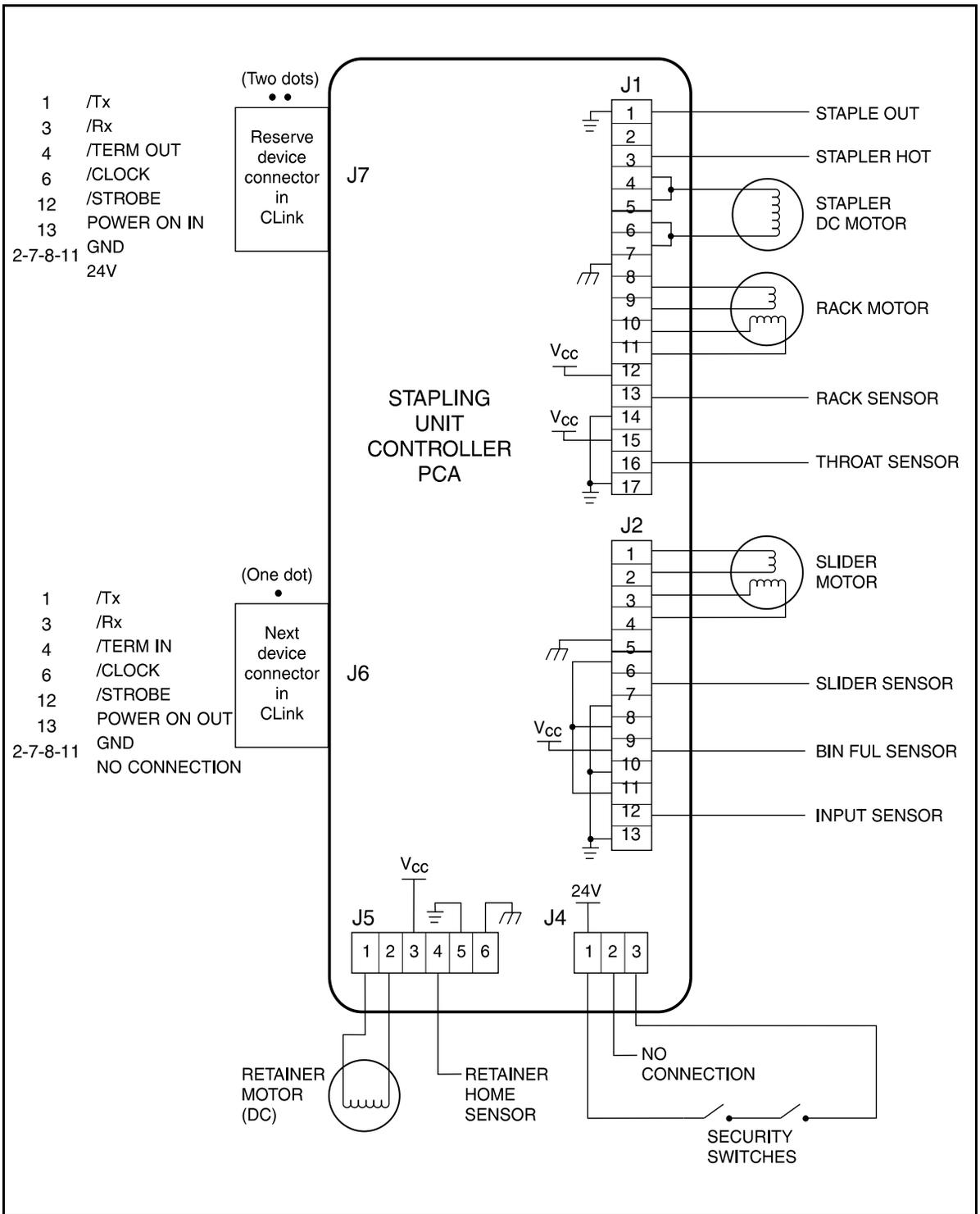
Figure 7-40 Stapling Unit Controller PCA Main Wiring Diagram
