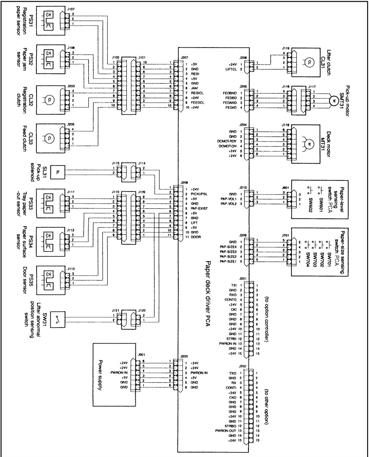
Figure 7-38 2000-Sheet Input Unit Main Wiring Diagram
