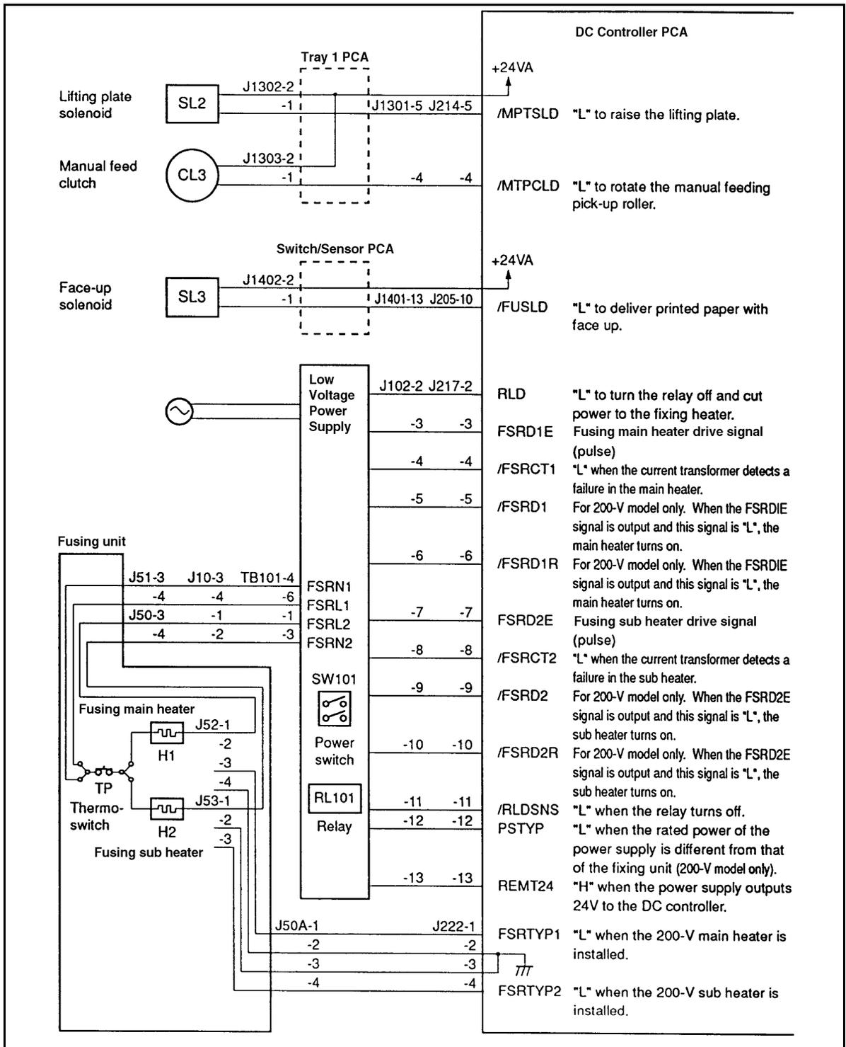
Figure 7-34 DC Controller Inputs and Outputs (5 of 5)
