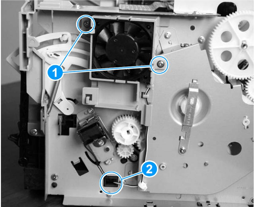
**Figure 72.** Removing the fan (2 of 2)
