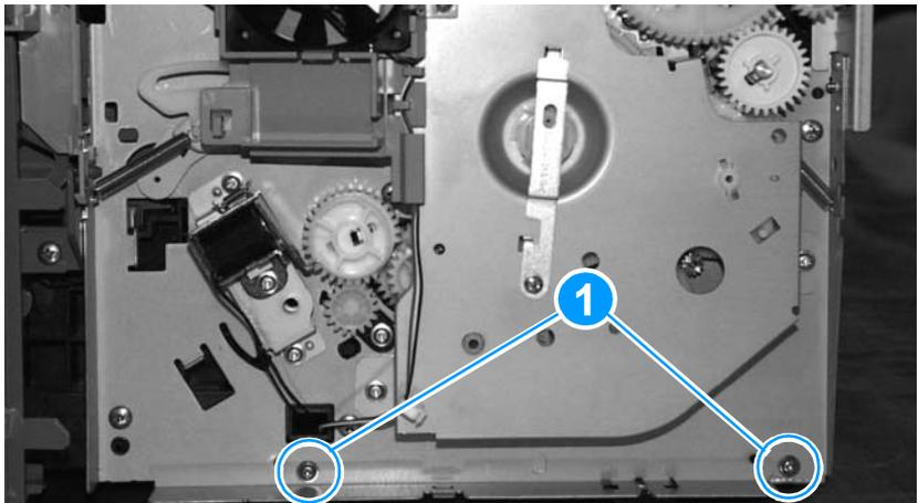
**Figure 87.** Removing the ECU pan (3 of 5)
