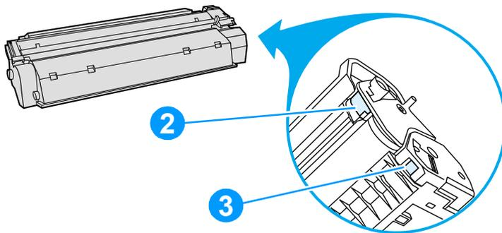
**Figure 97.** Print cartridge high-voltage connection points (left side)
