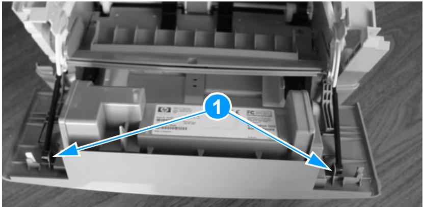
**Figure 48.** Removing the print cartridge door (1 of 2)
