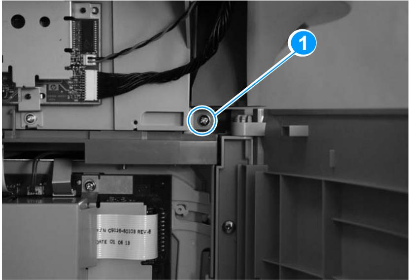
**Figure 28.** Separating the scanner from the printer (2 of 4)
