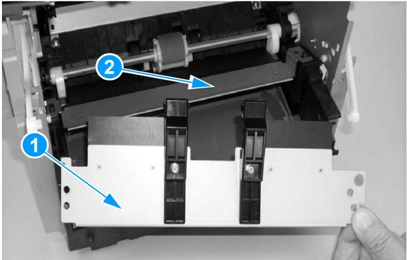
**Figure 75.** Removing the pickup assembly plate (3 of 3)
