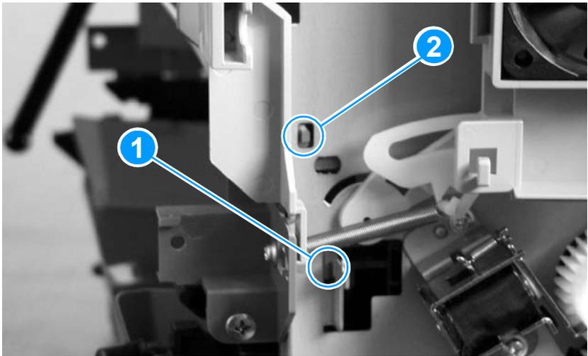
**Figure 54.** Removing the front guide assembly (2 of 3)
