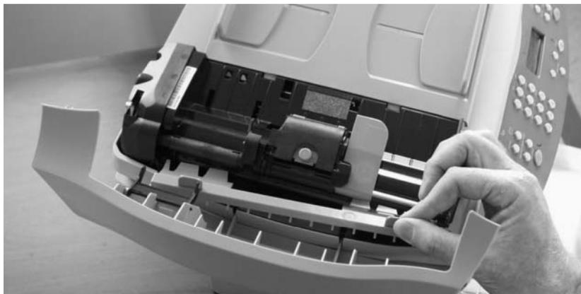
**Figure 32.** Removing the document feed guide (1 of 2)
