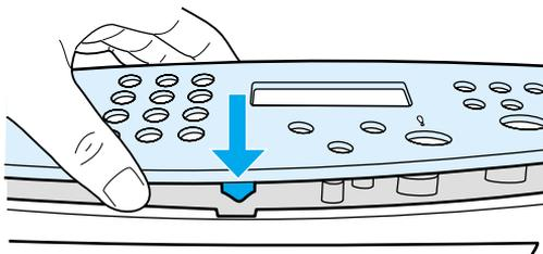
**Figure 36.** Reinstalling the control panel bezel (1 of 2)
