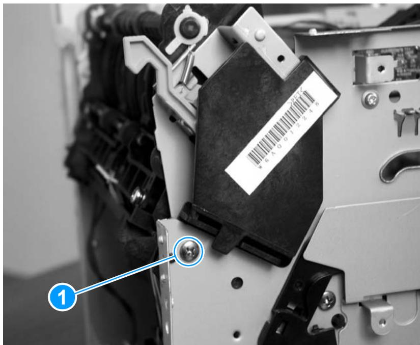
**Figure 64.** Removing the fuser assembly (3 of 4)
