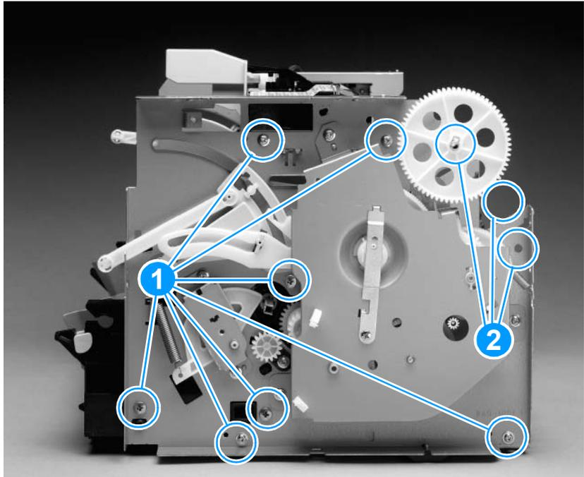
**Figure 82.** Removing the right plate assembly (2 of 2)
