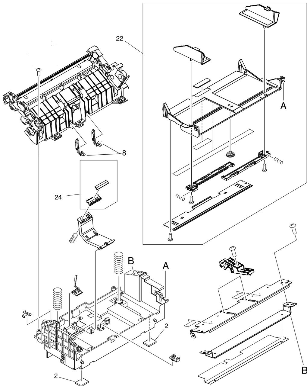
**Figure 119.** Paper pickup assembly (2 of 2)
