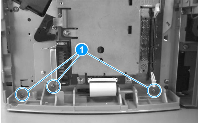
**Figure 84.** Removing the left bottom frame support
