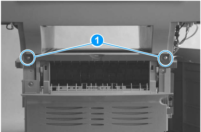
**Figure 29.** Separating the scanner from the printer (3 of 4)
