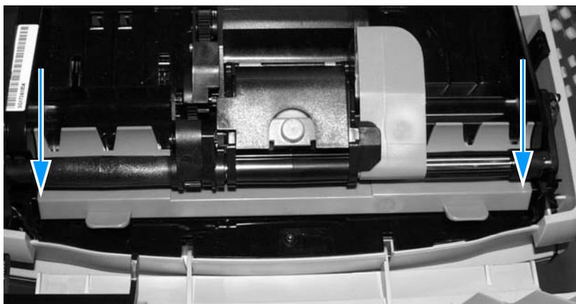
**Figure 33.** Removing the document feed guide (2 of 2)
