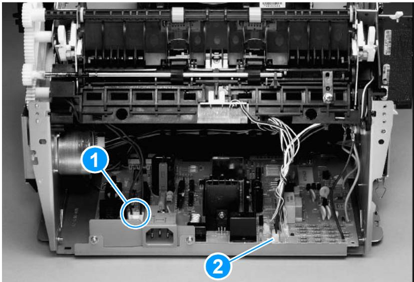
**Figure 95.** Locating connectors for the heating element check
