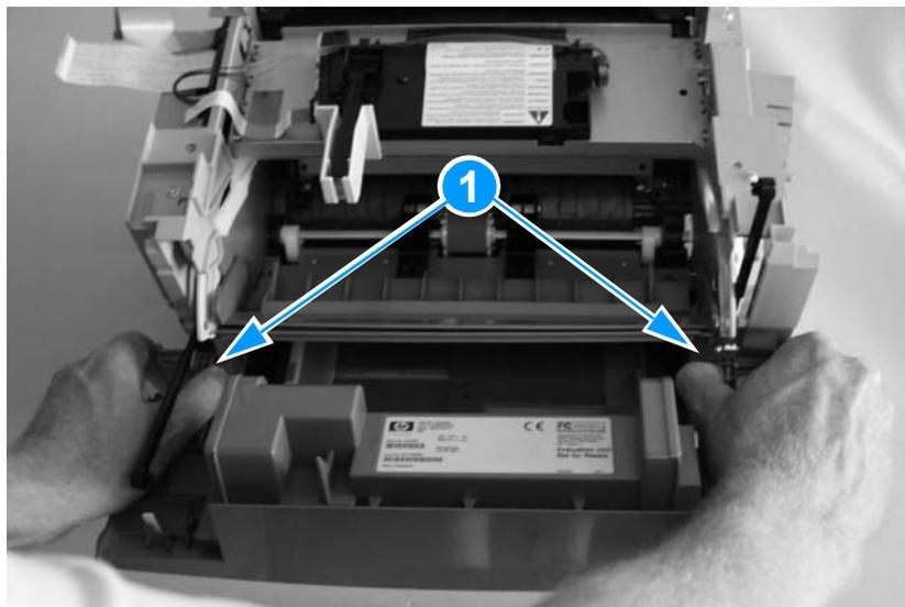
**Figure 49.** Removing the print cartridge door (2 of 2)
