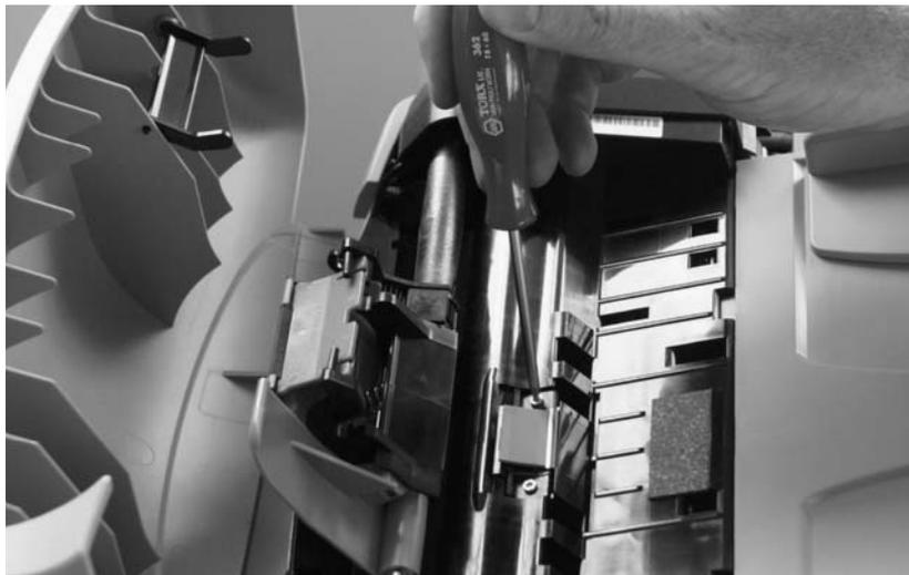
**Figure 34.** Removing the ADF separation pad
