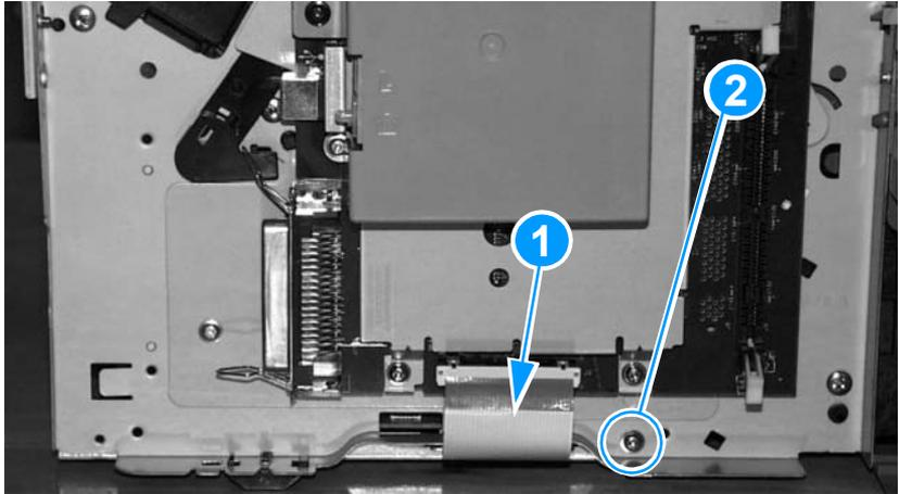
**Figure 86.** Removing the ECU pan (2 of 5)
