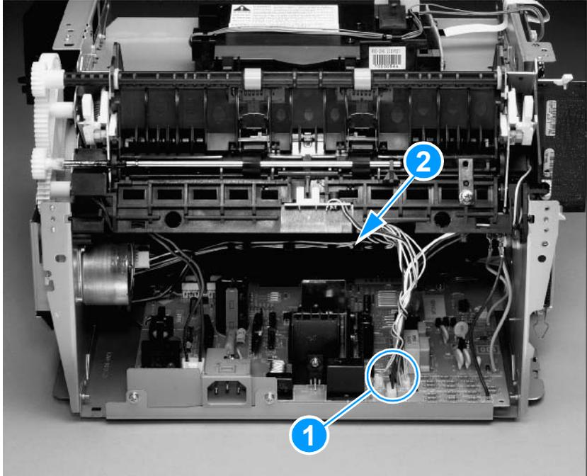
**Figure 69.** Removing the solenoid (1 of 2)
