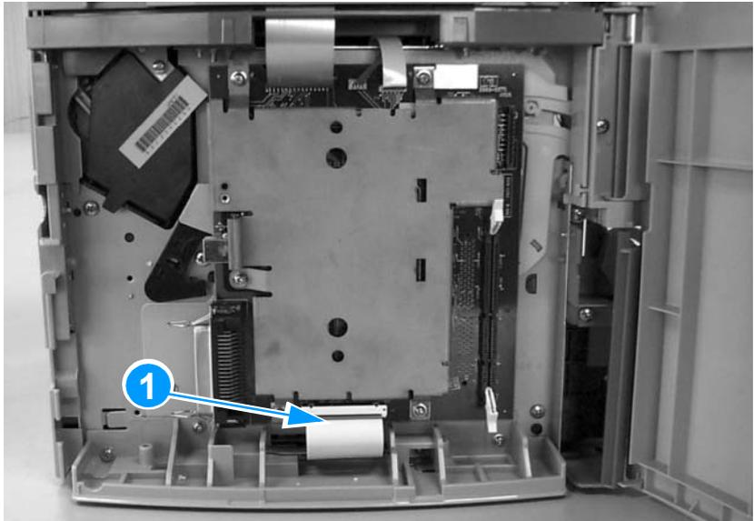
**Figure 59.** Removing the formatter (1 of 3)
