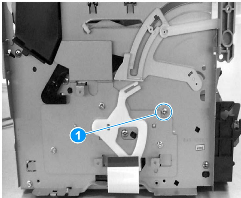
**Figure 73.** Removing the pickup assembly plate (1 of 3)
