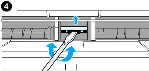
4 To pry the separation pad up from the spring-loaded base, insert a flat-edged screwdriver in the slot under the separation pad and twist until the tabs are free.
