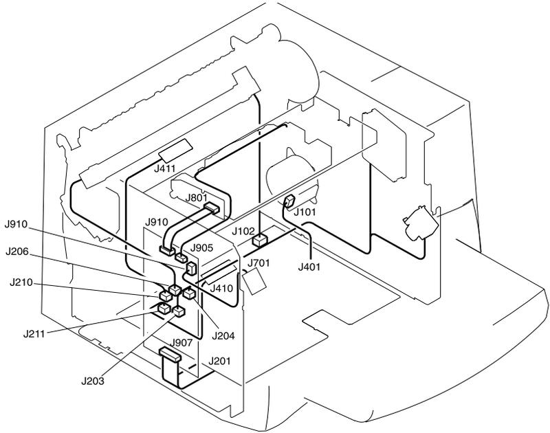
**Figure 108.** Locations of printer connectors
