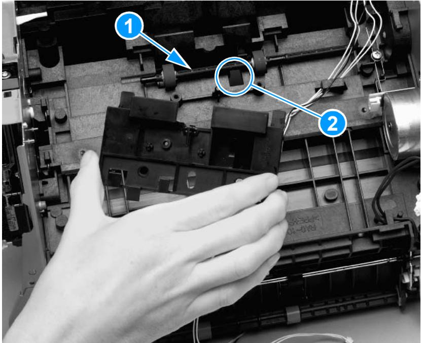
**Figure 91.** Removing the paper-feed assembly (2 of 4)
