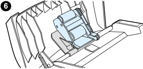
**6** To check for proper installation, lift the green lever until it remains open. The new pickup roller assembly should be secured to the lever assembly and should not fall out.
