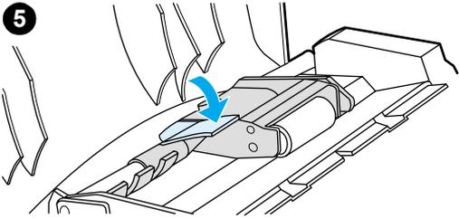
**5** Lower the green lever with the flat green part fitting in between the rollers. Press down on the green lever until the assembly snaps into place.
