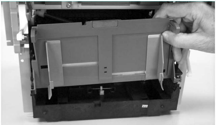
**Figure 78.** Removing the paper lift-plate assembly (3 of 3)
