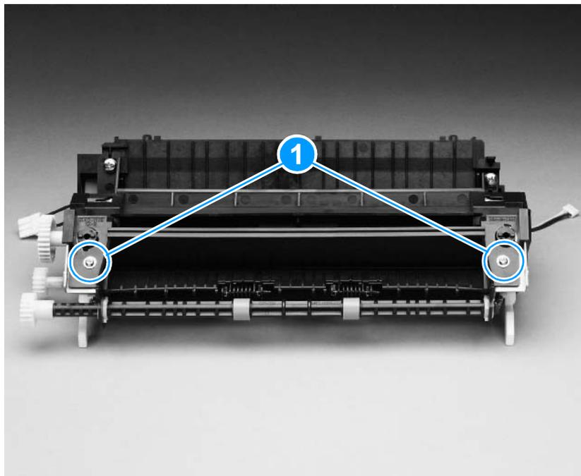
**Figure 66.** Removing the output rollers (1 of 2)
