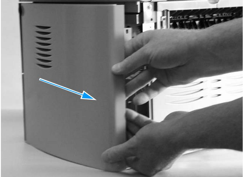
**Figure 24.** Removing the right side cover (3 of 3)
