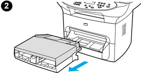
If the input tray feeds more than one page at a time, you might have to replace the printer separation pad. Recurring feed problems indicate that the printer separation pad is worn.
