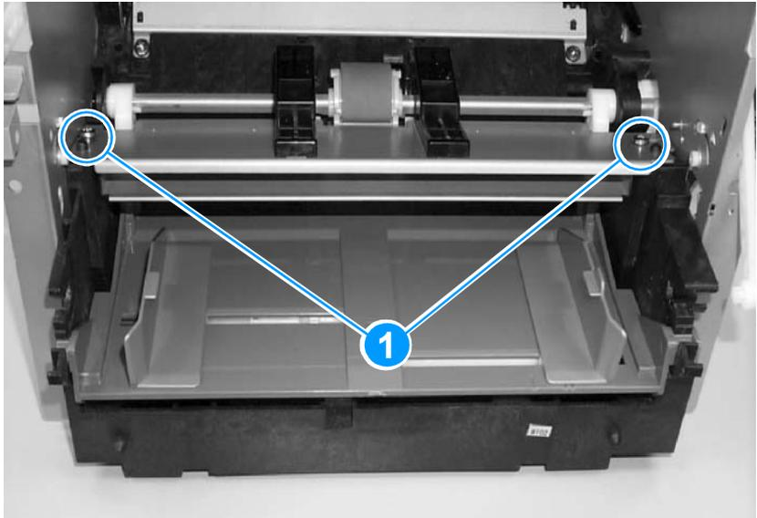
**Figure 74.** Removing the pickup assembly plate (2 of 3)
