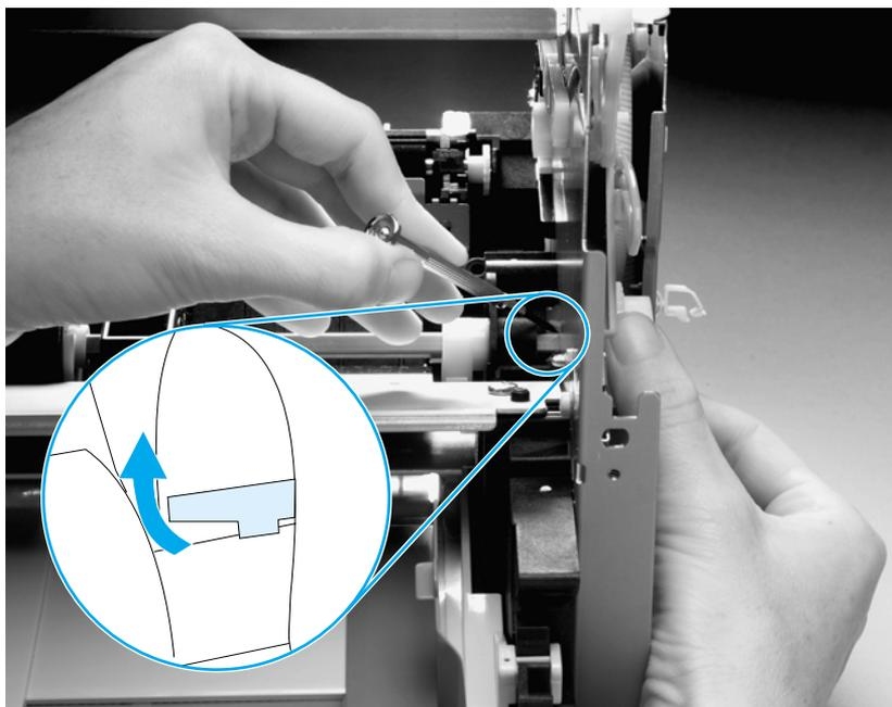
**Figure 81.** Removing the right plate assembly (1 of 2)
