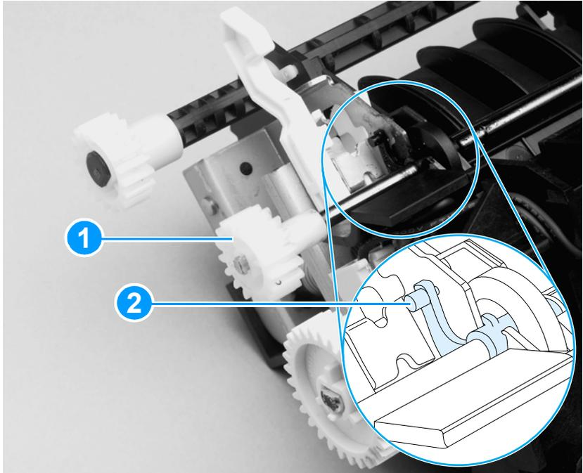
**Figure 67.** Removing the output rollers (2 of 2)
