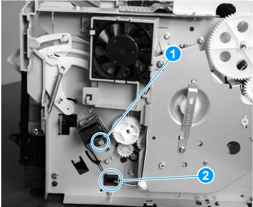
**Figure 70.** Removing the solenoid (2 of 2)
