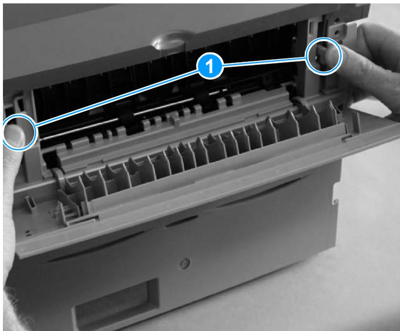
**Figure 46.** Removing the back cover (2 of 2)
