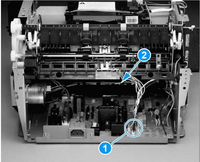
**Figure 71.** Removing the fan (1 of 2)
