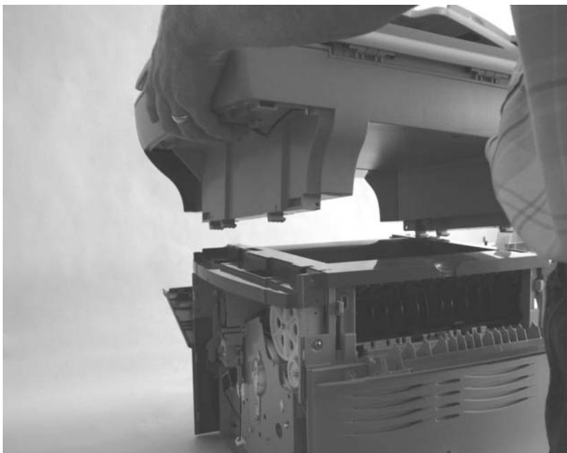
**Figure 30.** Separating the scanner from the printer (4 of 4)
