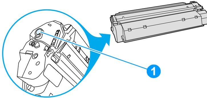
**Figure 96.** Print cartridge high-voltage connection points (right side)
