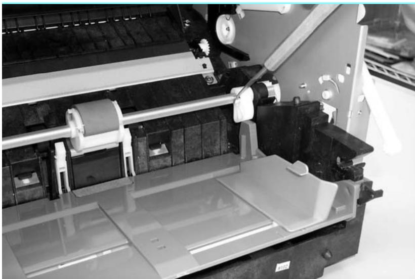
**Figure 76.** Removing the paper lift-plate assembly (1 of 3)
