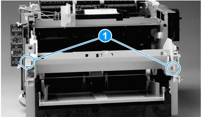
**Figure 53.** Removing the front guide assembly (1 of 3)
