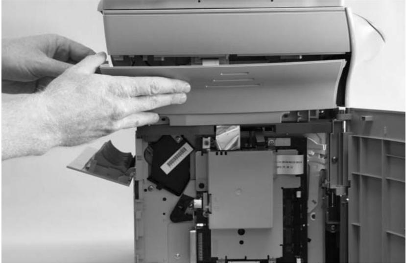
**Figure 26.** Removing the left scanner cover
