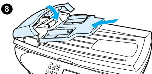
**8** Lower the green lever assembly and close the ADF lid. Reinstall the input tray.
