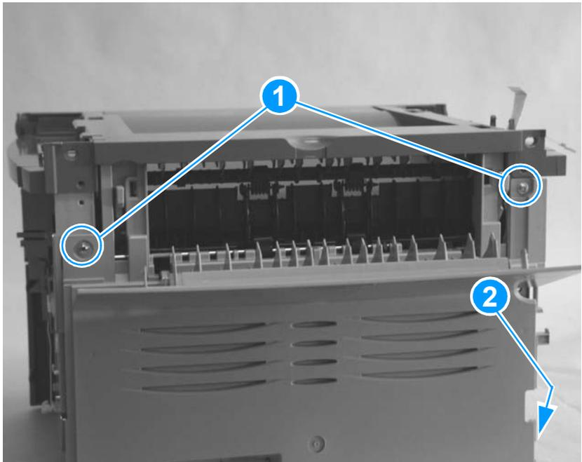
**Figure 45.** Removing the back cover (1 of 2)
