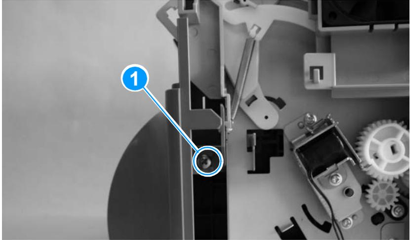
**Figure 50.** Removing the front cover (1 of 2)
