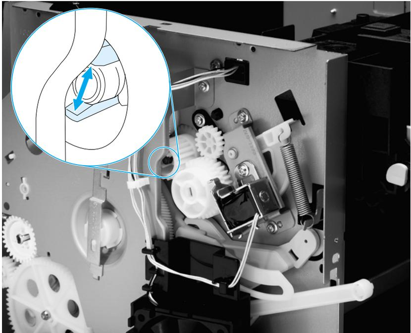
**Figure 92.** Removing the paper-feed mechanism (3 of 4)
