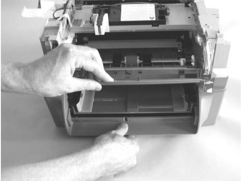
**Figure 52.** Removing the front cover (2 of 2)
