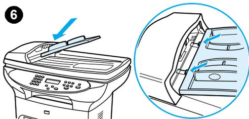
6 Install the ADF input tray by aligning the two tabs on the input tray with the two grooves in the ADF lid and sliding the tray into the grooves until it snaps into place.
