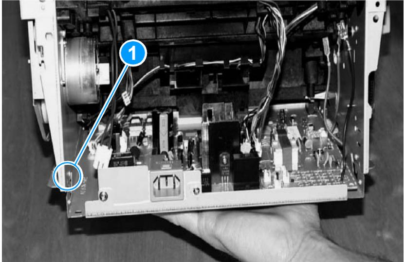
**Figure 88.** Removing the ECU pan (4 of 5)
