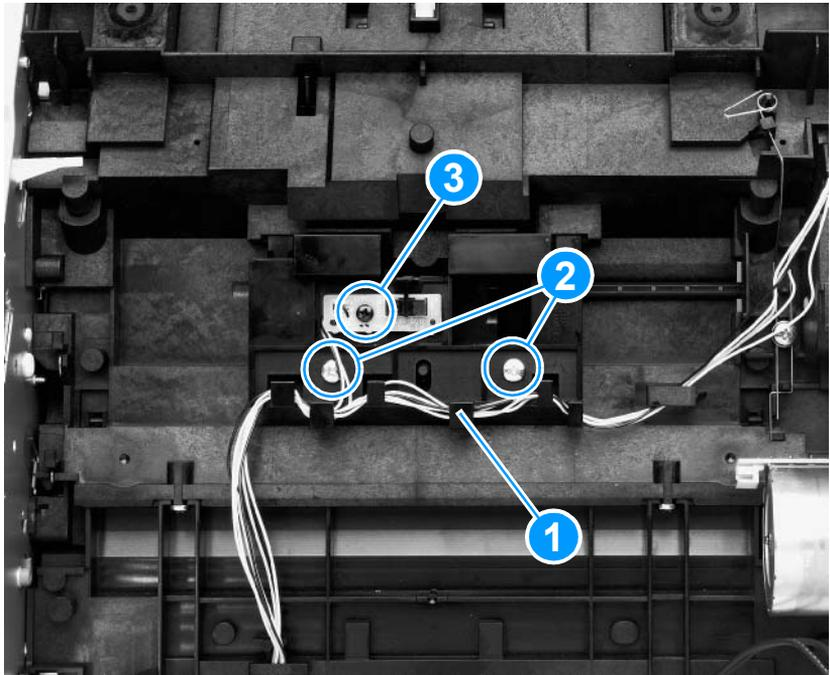
**Figure 90.** Removing the paper-feed assembly (1 of 4)
