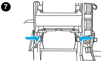
**7** Make sure that both sides of the assembly are secured by the green hooks.
