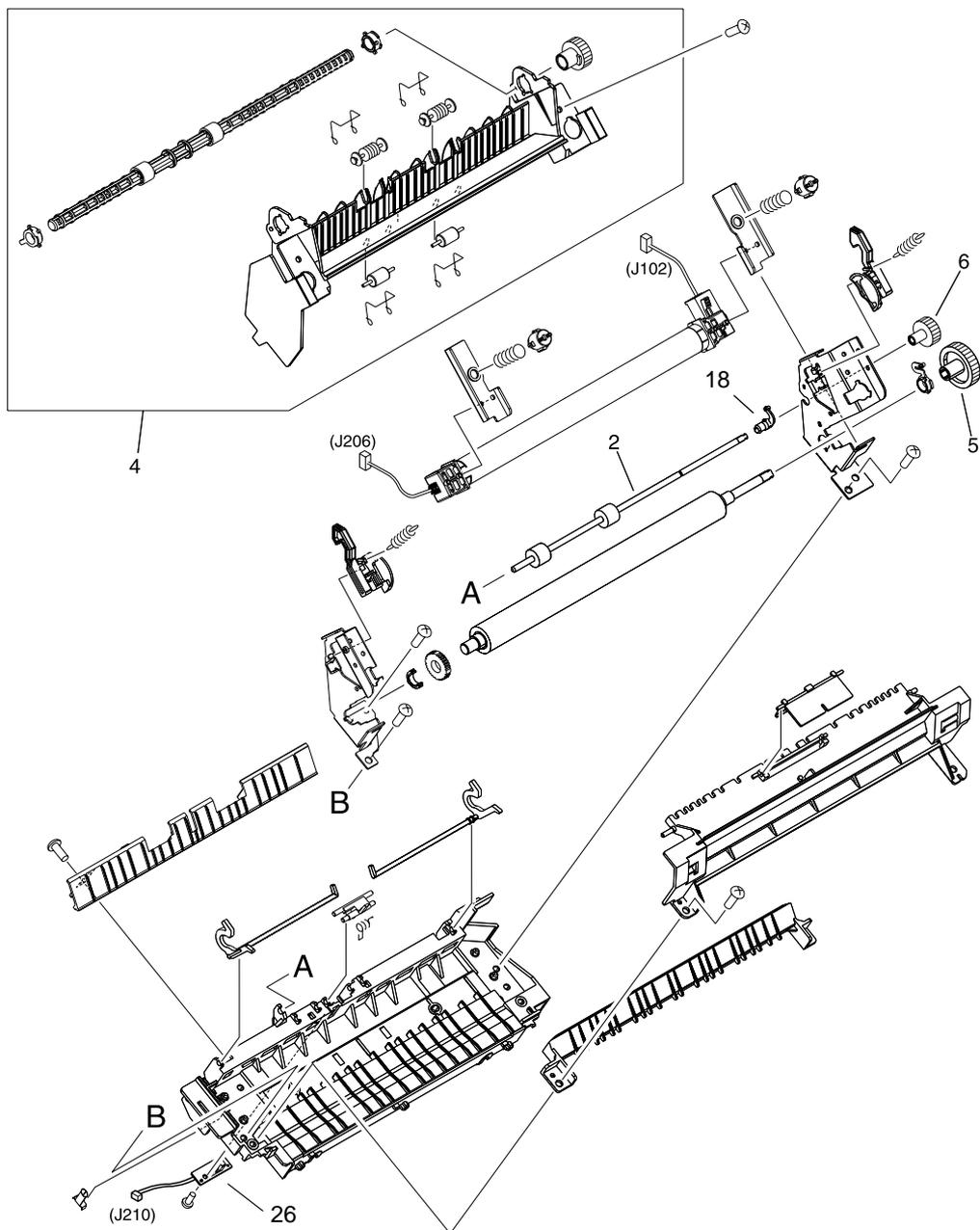
**Figure 120.** Fuser assembly
