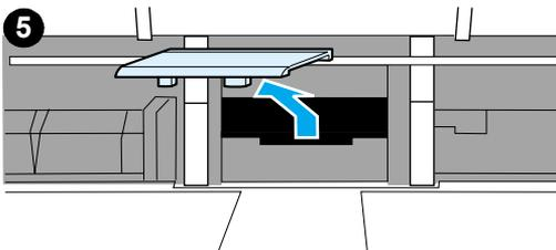
5 Reach in through the input tray opening, push the spring-loaded base down with one hand, and pull the separation pad up with the other hand.
