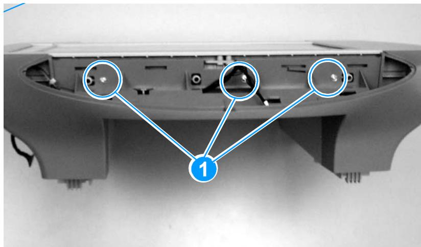
**Figure 39.** Removing the control panel chassis (1 of 2)
