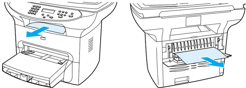
**Figure 9.** Output bin and straight-through output path
