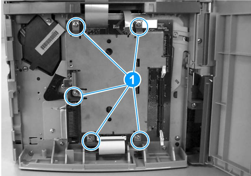
**Figure 60.** Removing the formatter (2 of 3)
