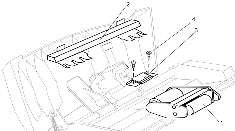
**Figure 111.** ADF rollers and separation pad
