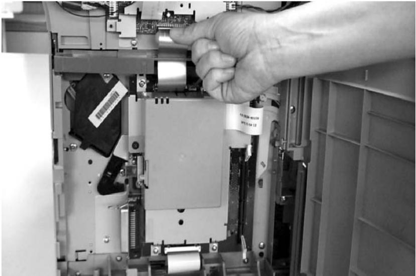
**Figure 27.** Separating the scanner from the printer (1 of 4)
