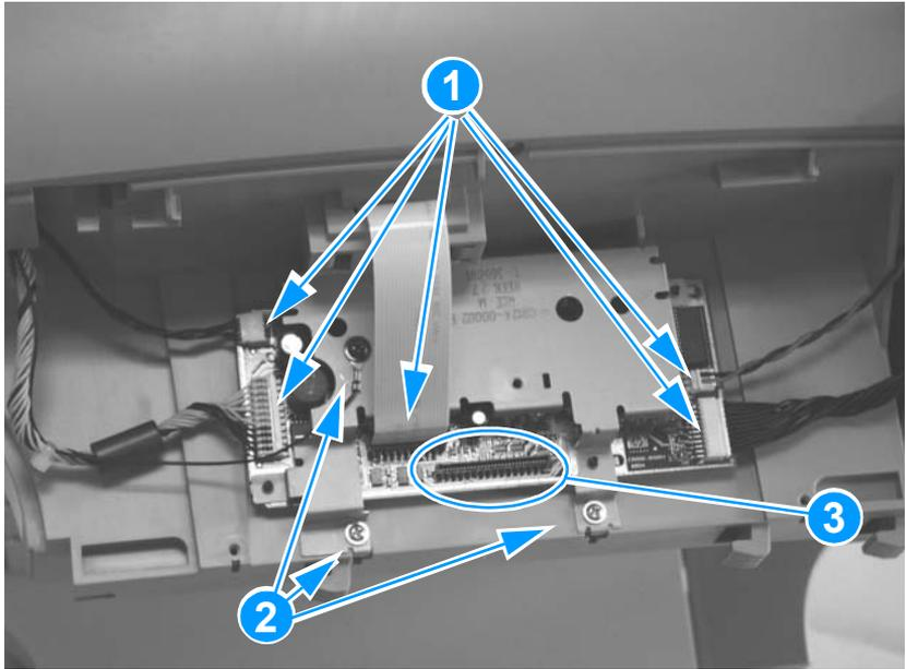
**Figure 41.** Removing the scanner formatter
