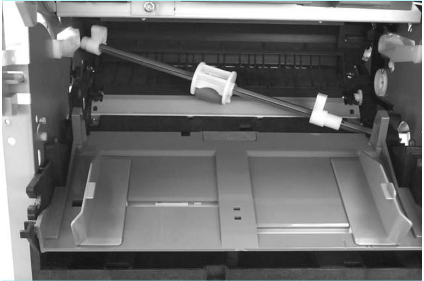
**Figure 77.** Removing the paper lift-plate assembly (2 of 3)
