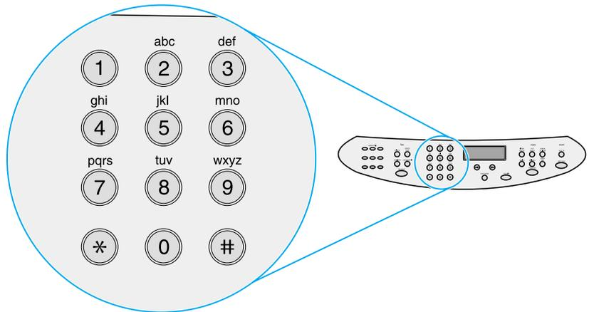
**Figure 6.** Alphanumeric controls
