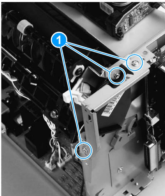
**Figure 63.** Removing the fuser assembly (2 of 4)
