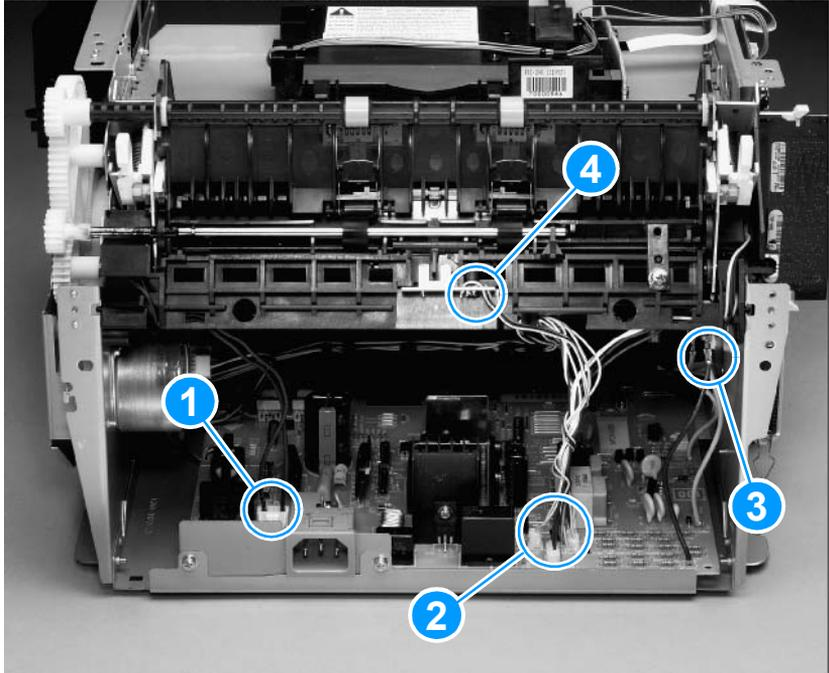
**Figure 65.** Removing the fuser assembly (4 of 4)
