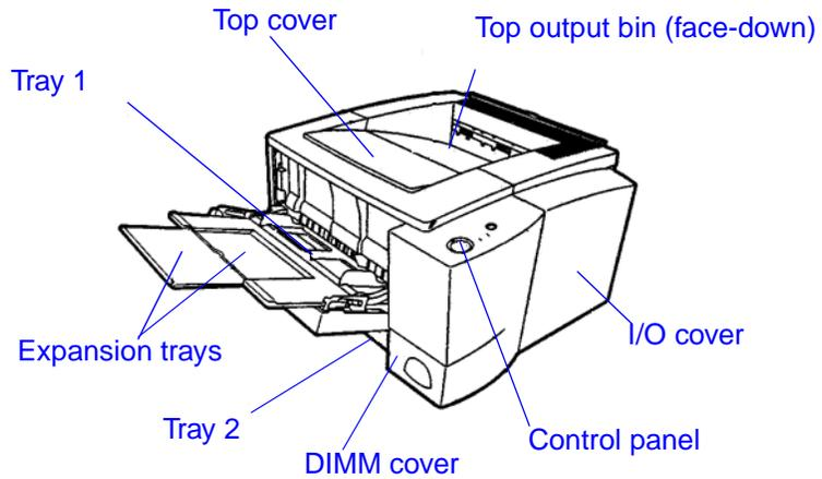
Figure 1-3 External Assembly Locations (2 of 4)
