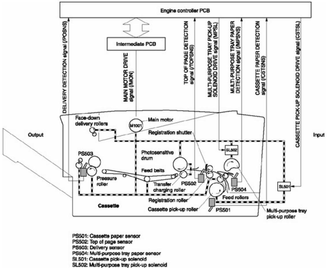
**Figure 6-7** Optional Tray 3 Paper Path, Sensors, and Signal
