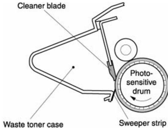
At the cleaning stage, the photosensitive drum's surface is prepared to hold an image. During printing, the drum rotates completely several times per printed page. Before forming the image for a given section of print, a cleaning blade removes toner from the previous rotation of the drum. The toner cartridge stores waste toner and prevents it from being used in later print jobs (see figure 5-9).
