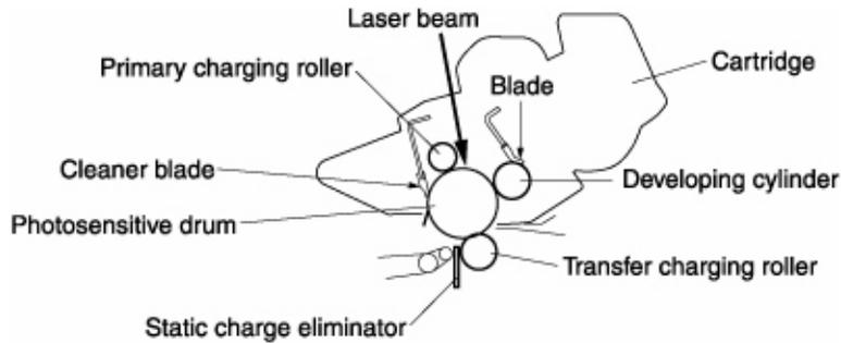
The toner cartridge contains the cleaning, conditioning, and developing stages of the image formation process. These components are subject to wear and are built into the replaceable toner cartridge. This eliminates the need for a service call when replacement is required.
