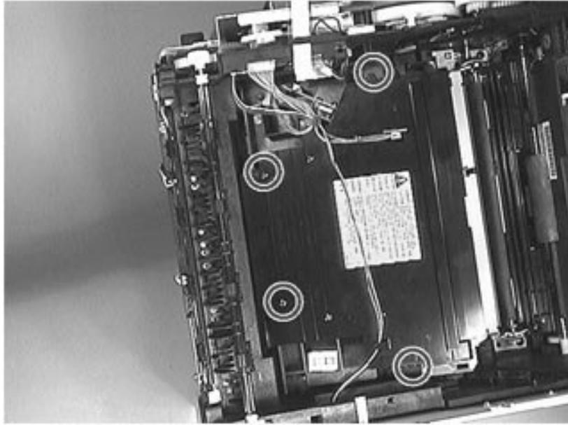
5 Lift the laser scanner assembly out of the printer.
