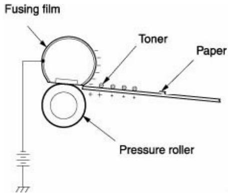
At the fusing stage, heat and pressure fuse the toner to the paper to produce a permanent image. The paper passes between a fusing film and a pressure roller. The fusing film melts the toner while the pressure roller compresses it into the paper.
