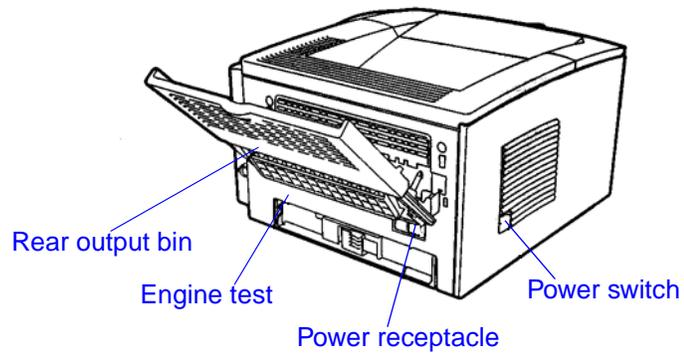
Figure 1-4 External Assembly Locations (3 of 4)
