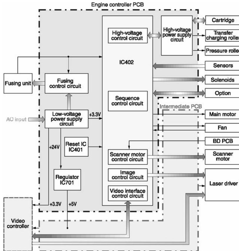
Specifically, the Engine Control System directly controls the following subsystems contained on the Engine Controller Assembly:
