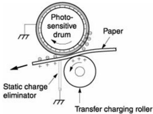
At the transferring stage, the toner image on the photosensitive drum's surface is moved to the paper. The transfer roller applies a positive charge to the back of the paper, causing the paper to attract the negatively charged toner on the drum's surface.
