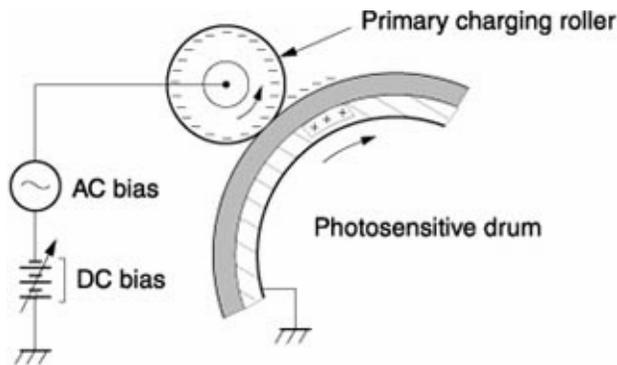
At the Conditioning Stage, the primary charging roller applies a uniform negative charge on the photosensitive drum's surface. The primary charging roller erases any residual charges and maintains a constant potential on the drum's surface. In addition, the primary charging roller creates a uniform negative potential on the drum's surface.
