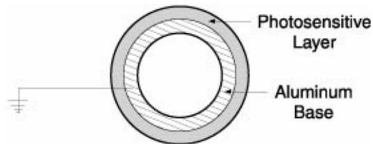
The photosensitive drum is the heart of the image formation system. This drum's special properties allow an image to form on the drum's surface and then transfer to paper. The drum is an aluminum cylinder coated with an organic-photoconductive material (OPC). The photosensitive drum's aluminum base is electrically connected to ground. The OPC material becomes electrically conductive when exposed to light. Areas not exposed to light remain nonconductive and maintain their negative charge.
