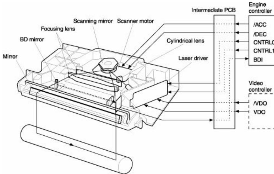
At the Laser Scanner, a laser beam focuses onto the photosensitive drum and discharges the drum's negative potential. This creates a latent electrostatic image, which later is developed into a visible image.
