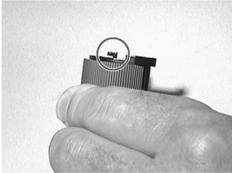
**Figure 7-118 Removing the Tray 1 Pickup Roller**
