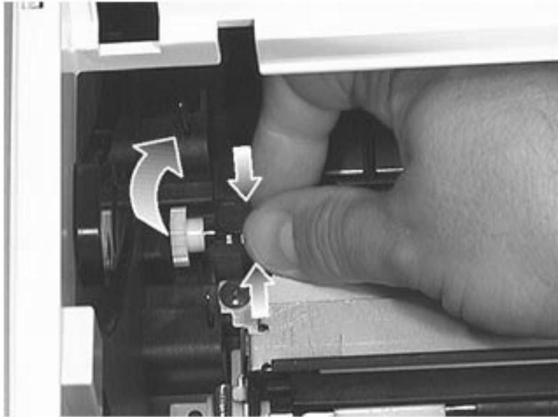
**Figure 7-6** Removing the Transfer Roller (2 of 2)
