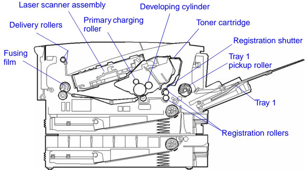
Figure 1-7 Internal Assembly Locations (2 of 2)
