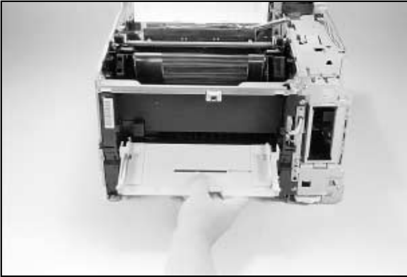
Figure 6-12 Rotate the Tray Down to Release the Hinge from its Slots
