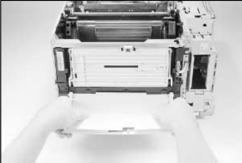
Figure 6-10 Removing the MP Tray Door
