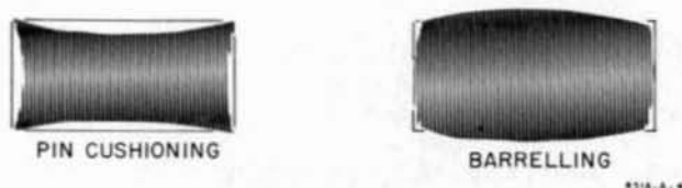
Figure 5-4. Pin-cushioning and Barrelling Defined
