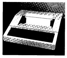
to a unique head design, adjustment for forms thickness variations between .08mm (.003") and 43mm (.017") is usually not required. A lever adjustment on the print head carriage is provided to allow optimization of print quality on various forms.
