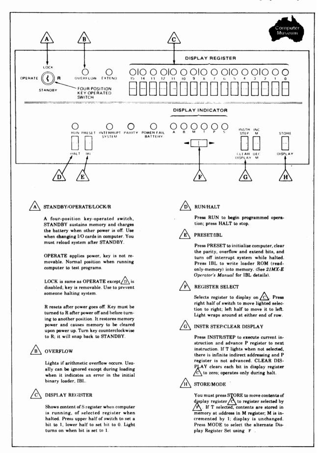
Figure 2-1. The 21MXE Front Panel
