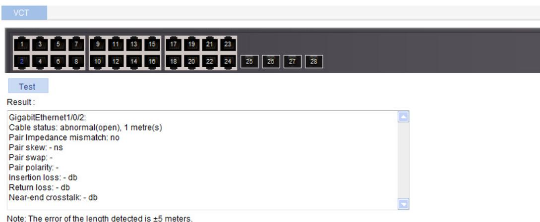
The result displays the cable status and length. The cable status can be normal, abnormal, abnormal (open), abnormal (short), or failure.
