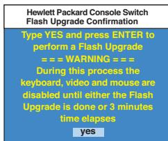
5. Using HyperTerminal to upgrade the FLASH code\*
