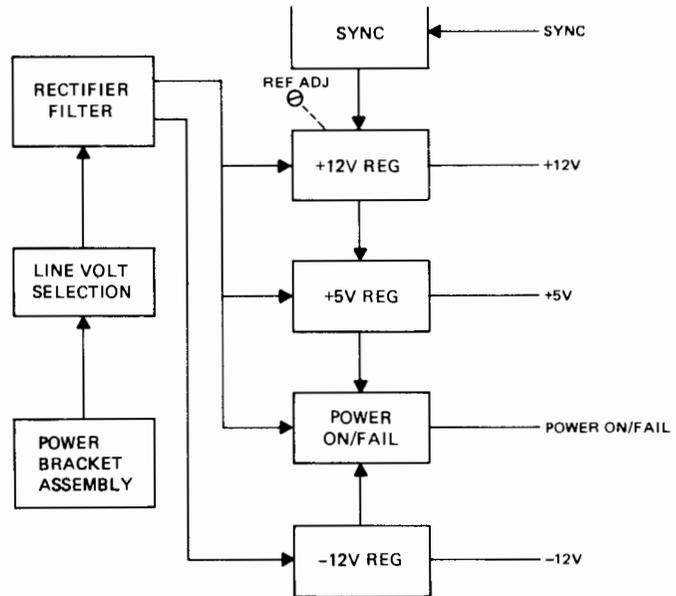
Figure 8-5. 2621A Power Supply, Simplified Block Diagram
