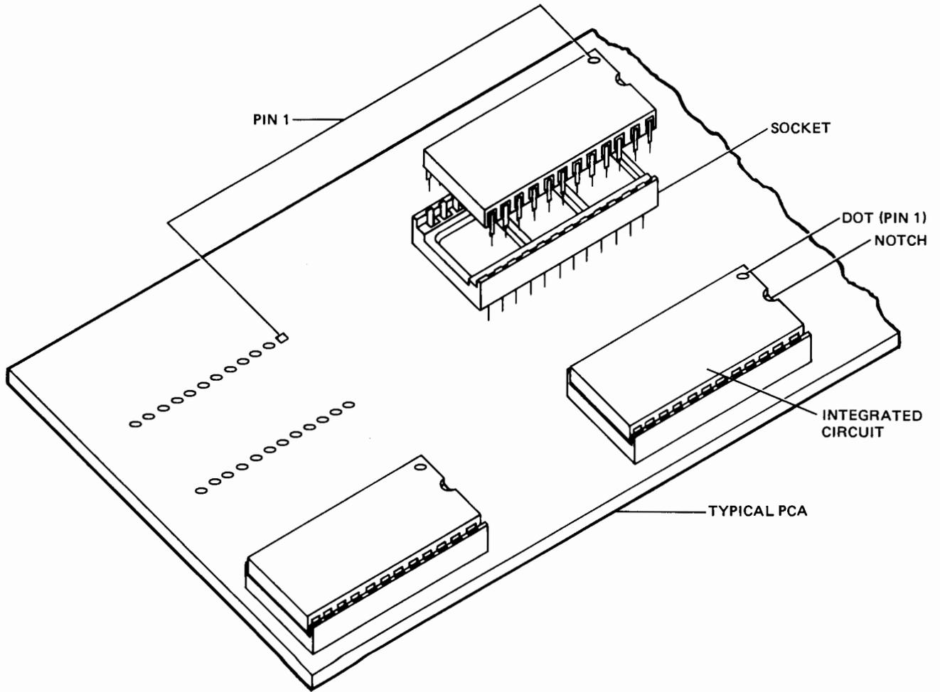
Figure 7-12. Installing an IC
