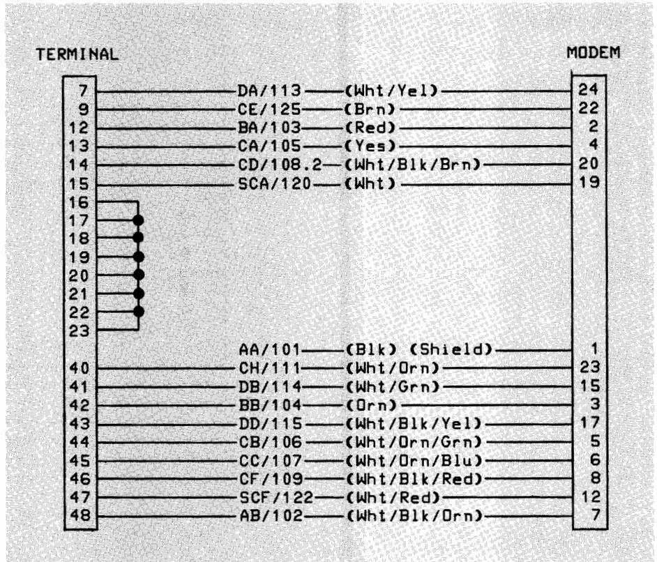
Figure 2-8. 13222M (European Modem) Cable Wiring
