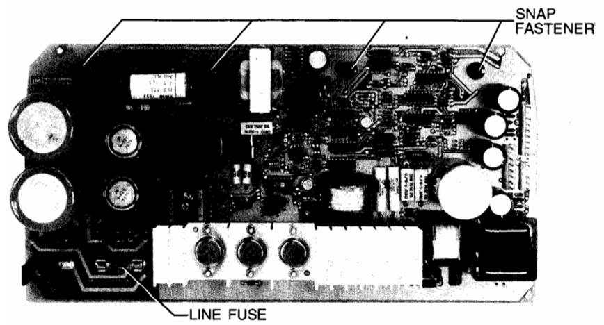
Figure 7-9. Power Supply PCA (2621P)
