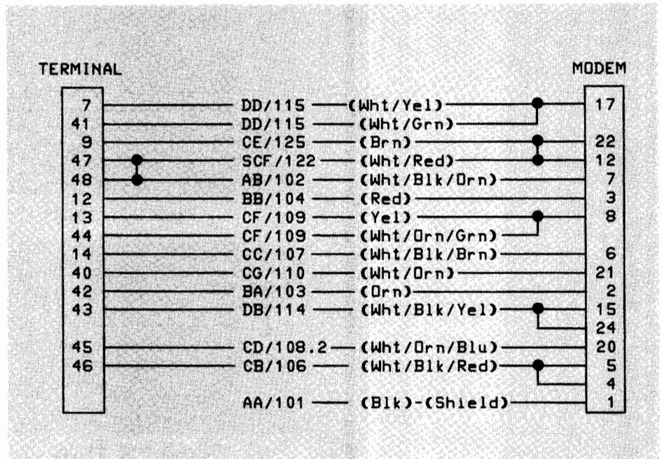
Figure 2-10. 13222W (HP 300) Cable Wiring
