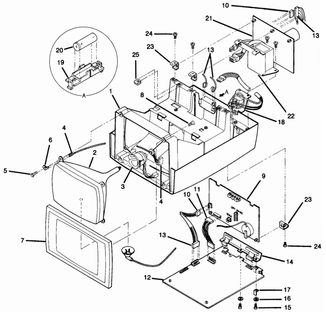
Figure 7-16A. Mainframe, Exploded View (2621A)
