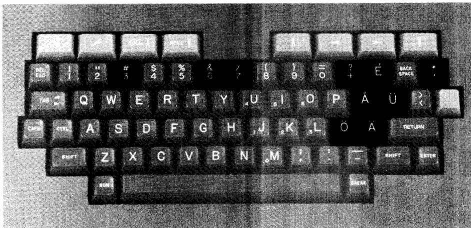
Figure 7-19. Swedish/Finnish Keyboard, Unique Keys
