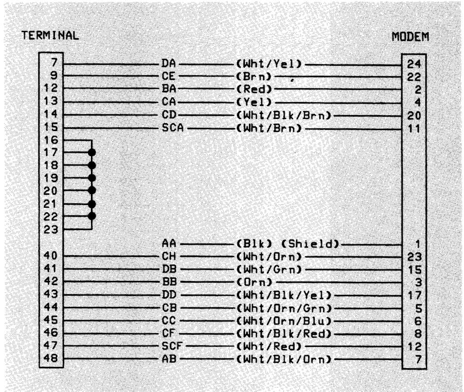
Figure 2-9. 13222N (U.S. Modem) Cable Wiring
