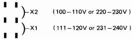
For example a 220 volt supply would use the J3 connector and the fuse would be placed across X2 connection (lower range).
