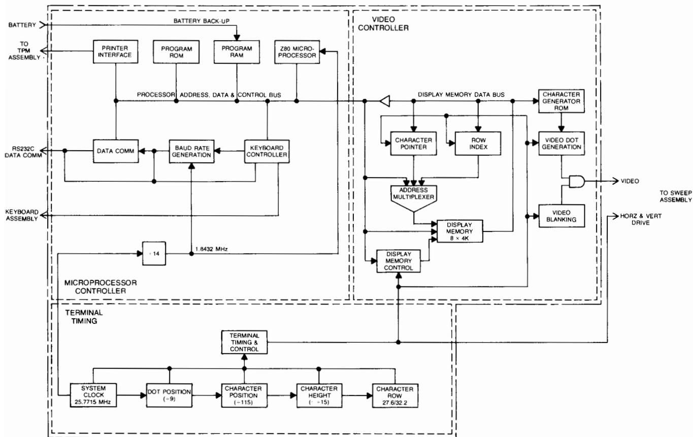
Figure 8-3. Processor PCA Block Diagram
