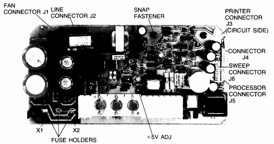
Figure 2-6. 2621P Power Supply PCA
