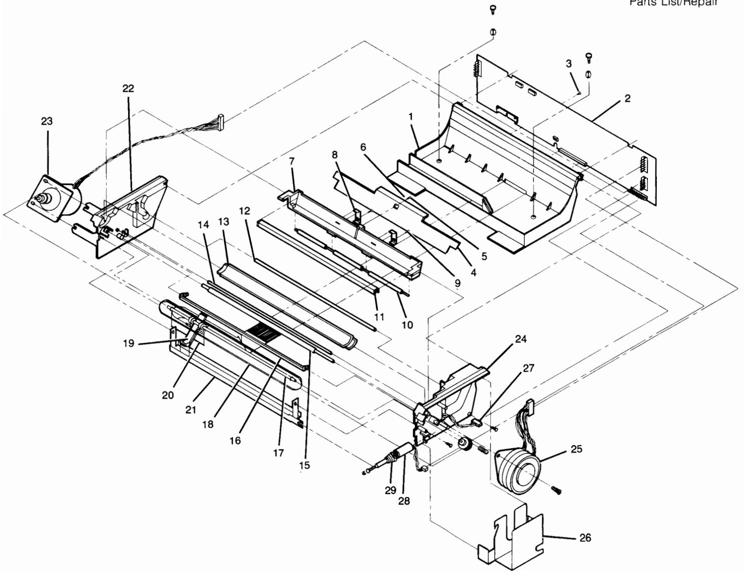
Figure 7-17. TPM, Exploded View
