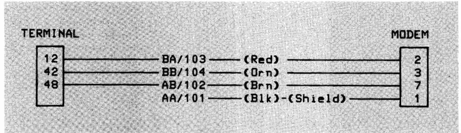
Figure 2-12. 13222Z (Three Wire/Female) Cable Wiring
