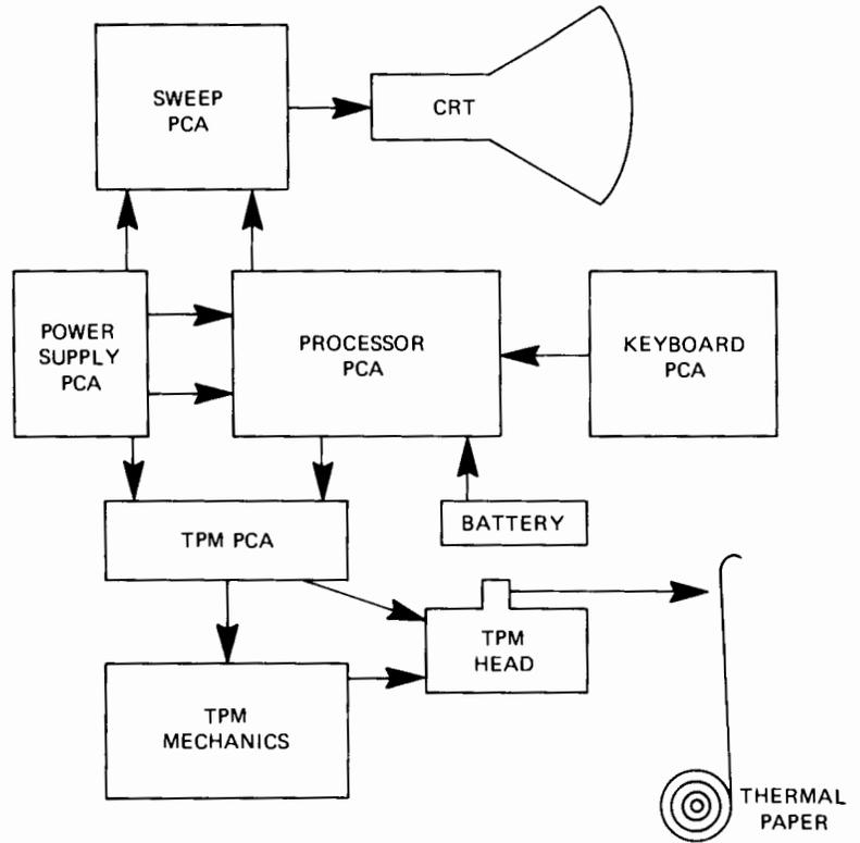
Figure 8-2. 2621P Simplified Block Diagram
