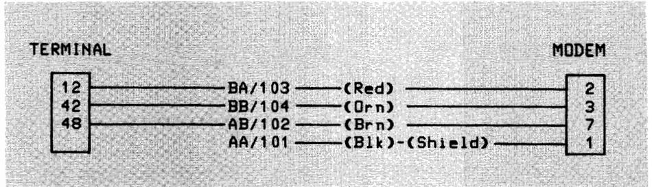
Figure 2-11. 13222Y (Three Wire/Male) Cable Wiring
