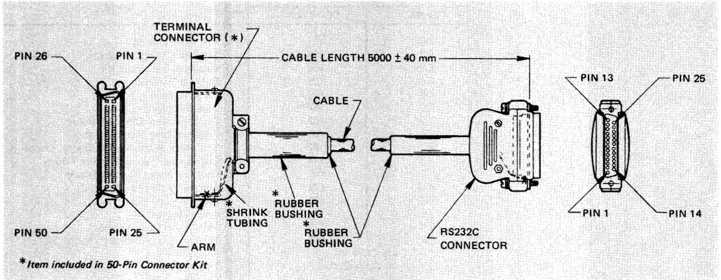
Figure 2-13. Cable Fabrication
