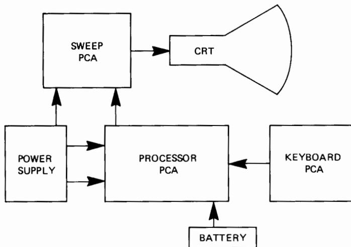
Figure 8-1. 2621A Simplified Block Diagram
