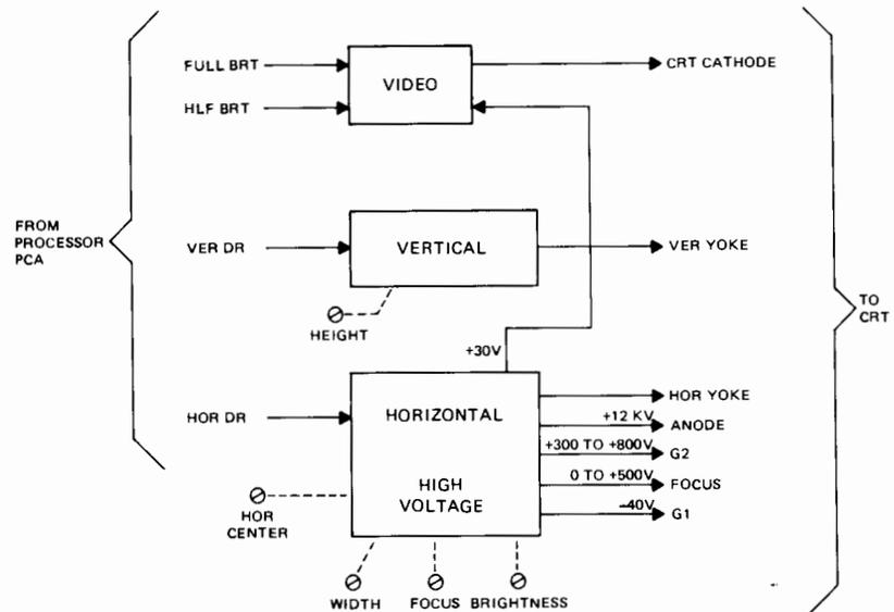
Figure 8-4. Sweep PCA, Simplified Block Diagram
