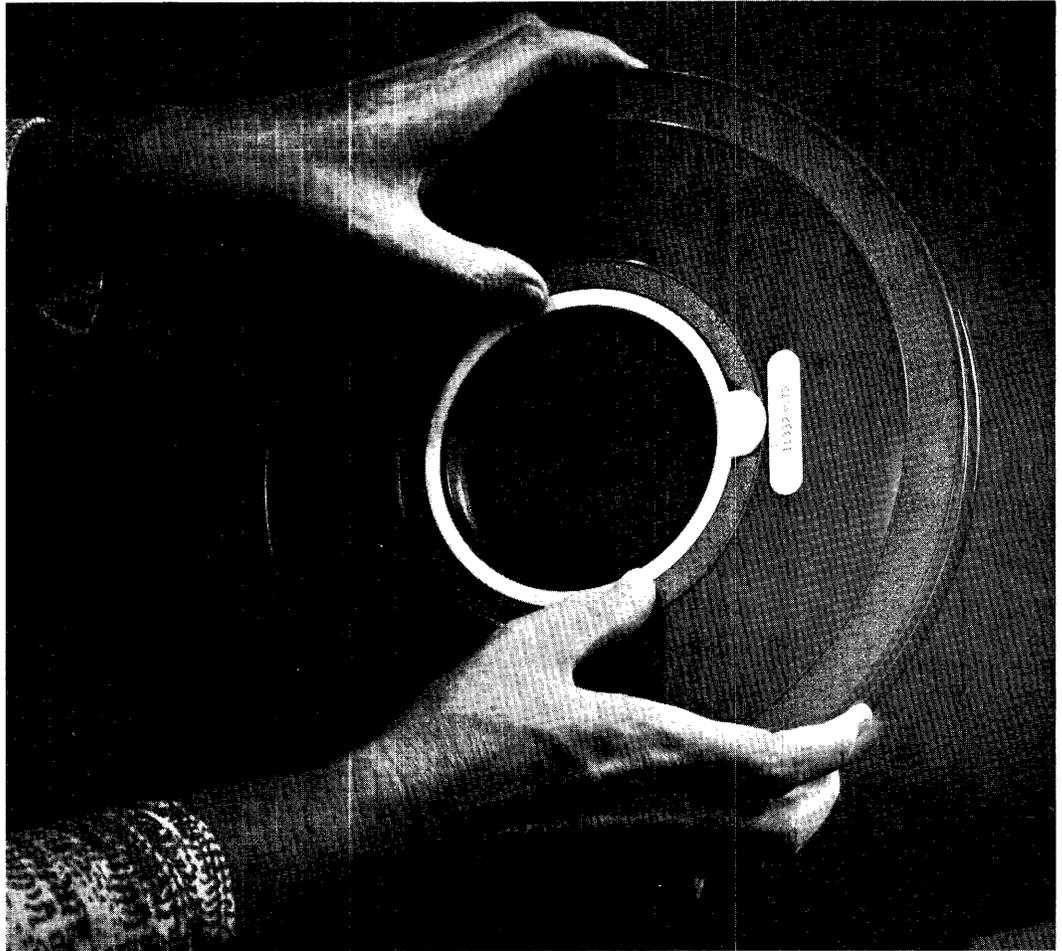
**Figure 2-2, Write Enable Ring**
