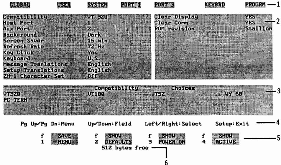
Figure 2-1. Format of Setup Menus
