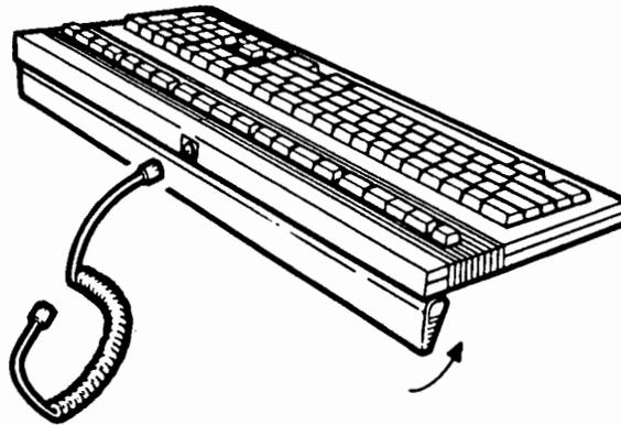
**Figure 1-4. Keyboard Cord Attachment and Angle Adjustment**
