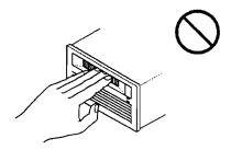
Do not restrain the cassette when pushing it into the drive. This may cause it to jam in the mechanism.
