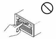
2 Apply steady pressure with one finger on the back of the cassette until the auto-loading mechanism takes the cassette and loads it into the drive. If the cassette appears not to load correctly, do not use additional force.
