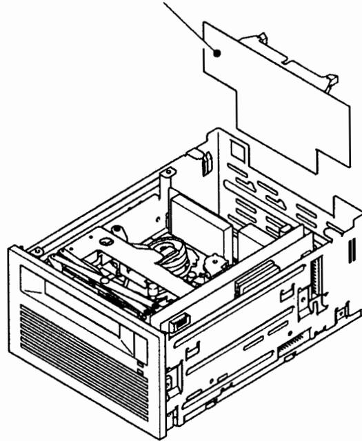
To remove the HP-IB Interface Driver PCA, proceed as follows:
