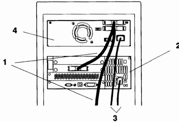
Figure 2-2. Connections to Host and Power
