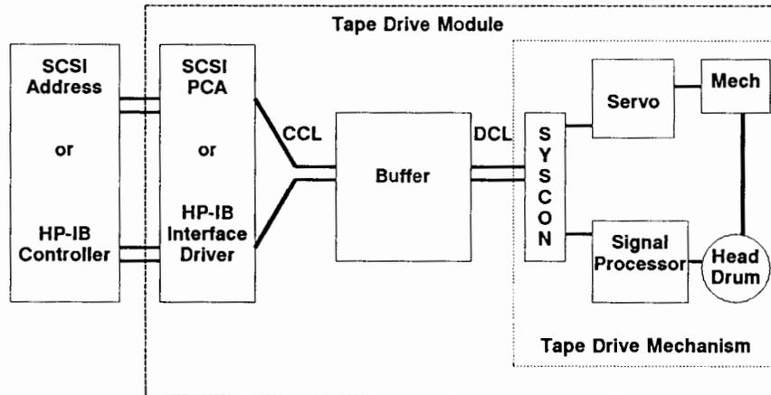
Figure 3-1. The Interface and Tape Drive Module of the 1300H and 1300S
