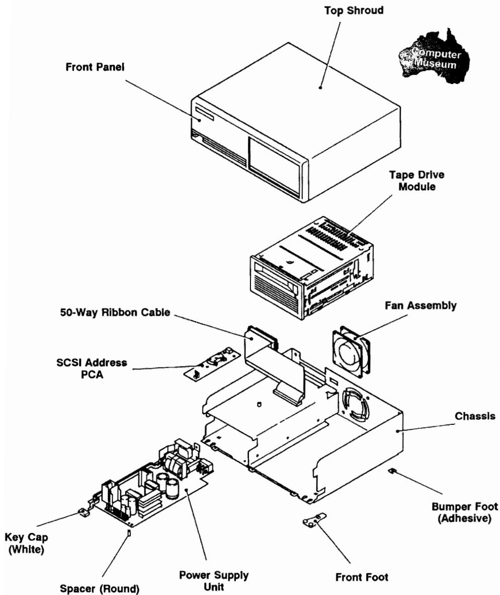
Figure 4-2. 1300S Exploded View
