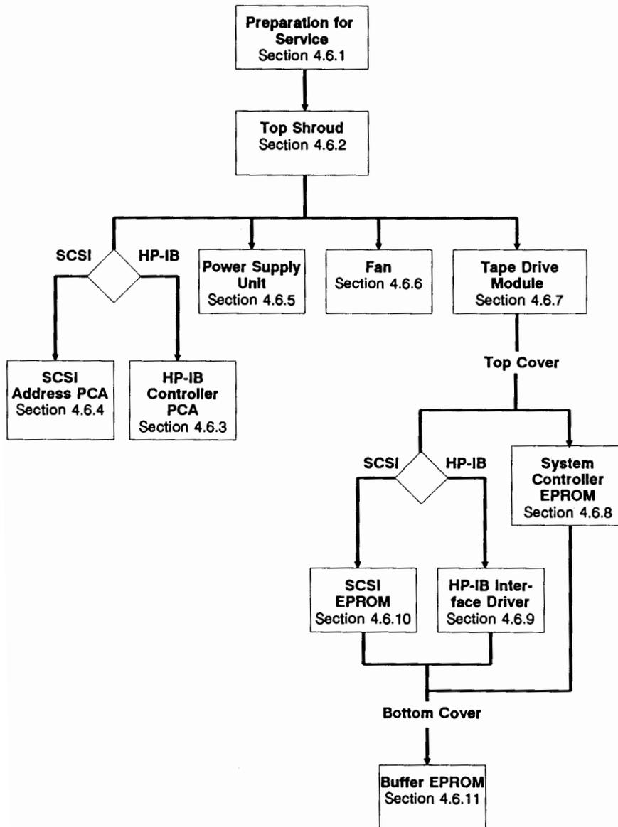
Figure 4-3. Order of Disassembly
