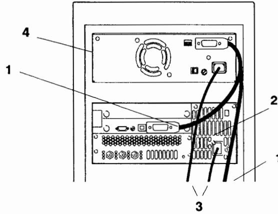
**Figure 2-1. Connections to Host and Power**
