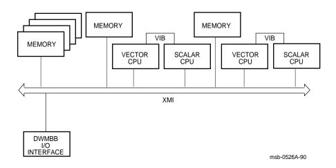
Figure 4–3: VAX 6000 Model 500 Vector Processing System
