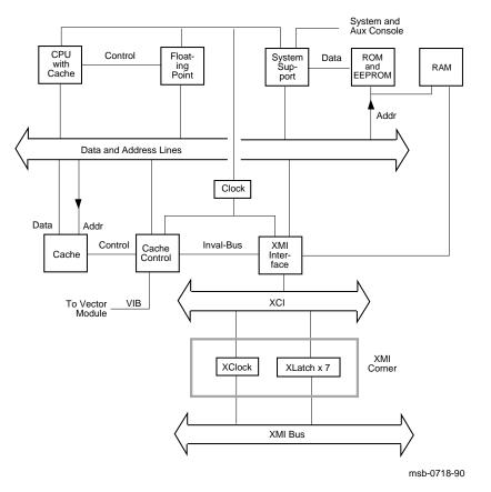
Figure 3–3: <REFERENCE>(xmp) Block Diagram
