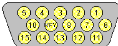
Figure 6-4. VGA Monitor Connector, (Female DB-15, as viewed from the rear of chassis).
