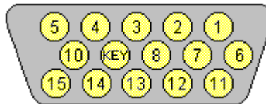
Figure 6–7. VGA Monitor Connector, (Female DB-15, as viewed from the rear of chassis).
