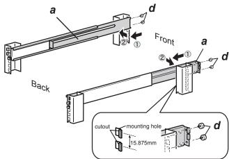
Slide the TeraStation into the rack until it clicks into place. Secure with hand screws *d*.
