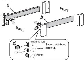
2 Slide the inner rack mounting brackets **a** into brackets **b** from the front, then secure them with hand screws **d**.
