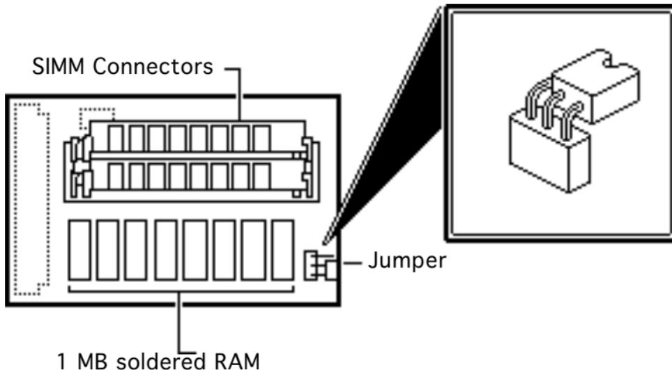
**Note:** The memory expansion board is an option for the Macintosh Classic only. It contains 1 MB of soldered RAM plus one pair of SIMM connectors. You can upgrade the system further by adding two 256K or two 1 MB SIMMs to the memory expansion board and moving the jumper. You must use 120-ns (or faster) SIMMs.
