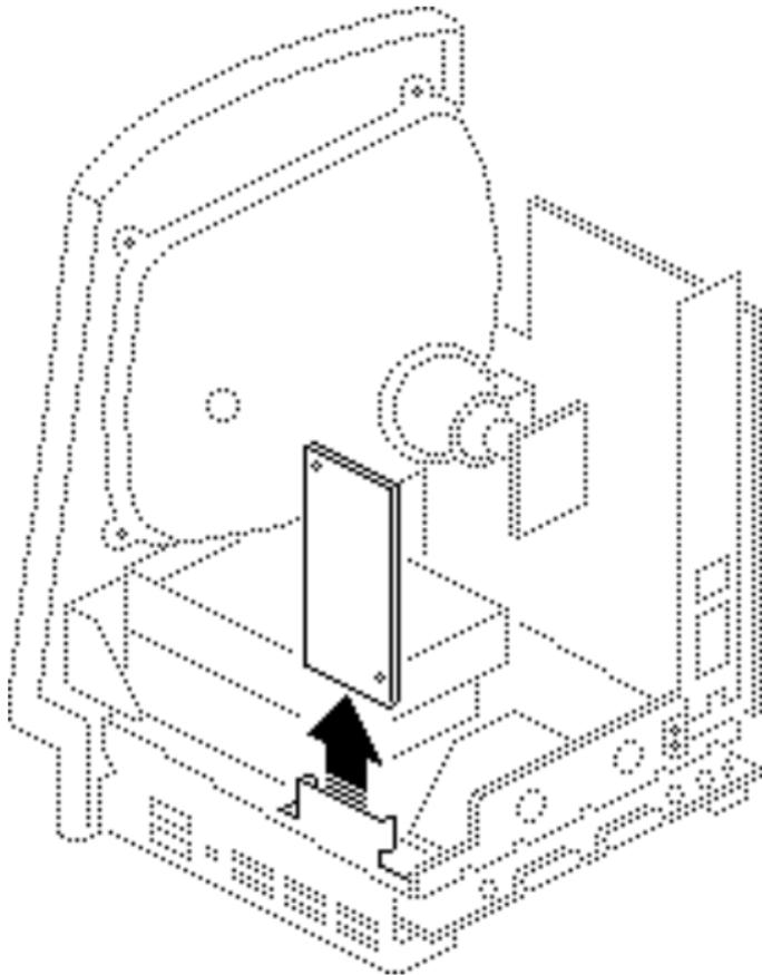
**Note:** The memory expansion board is an option for the Macintosh Classic only. It contains 1 MB of soldered RAM plus one pair of SIMM connectors.
