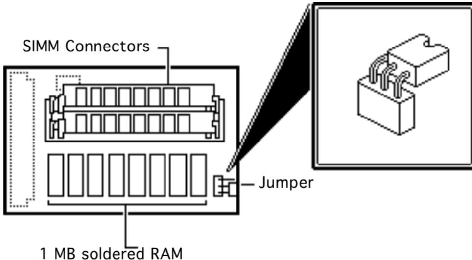
**Note:** Install the memory board without additional SIMMs for a 1 MB RAM upgrade. Install two 256K SIMMs onto the memory expansion board for a 2.5 MB RAM upgrade or two 1 MB SIMMs for a 4 MB RAM upgrade.
