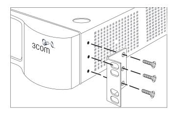
Figure 7 Fitting a bracket for rack mounting
